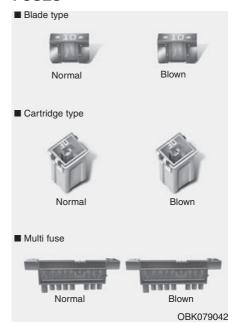
A vehicle's electrical system is protected from electrical overload damage by fuses.
