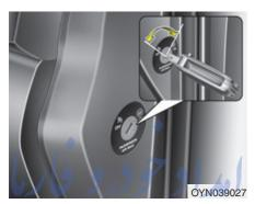
Passenger air bag "ON/OFF" switch (if equipped)
