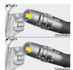
To flash the headlights, pull the lever towards you. It will return to the normal (low beam) position when released. The headlight switch does not need to be on to use this flashing feature.
