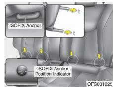
There are child restraint symbols located on the lower portion of each side of the rear seatbacks. These symbols indicate the position of the lower anchors for child restraints so equipped. Both rear outboard seats are equipped with a pair of ISOFIX anchorages as well as a corresponding top tether anchorage on the floor behind the rear seats. The ISOFIX anchorages are located between seat cushion and back rest, marked with the ISOFIX icon.
