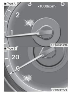
Your vehicle may be equipped with the ISG system, which reduces fuel consumption by automatically shutting down the engine, when the vehicle is at a standstill. (For example: red light, stop sign and traffic iam)
