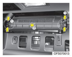
Remove the climate control air filter cover while pressing the lock on the right side of the cover.
