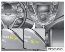
To deactivate or reactivate the passenger's front air bag:
