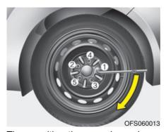
Then position the wrench as shown in the drawing and tighten the wheel nuts. Be sure the socket is seated completely over the nut. Do not stand on the wrench handle or use an extension pipe over the wrench handle. Go around the wheel tightening every nut following the numerical sequence shown in the image until they are all tight. Then double-check each nut for tightness. After changing wheels, we recommend that the system be checked by an authorized HYUNDAI dealer.
