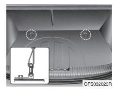
Securing a child restraint seat with "Tether Anchor" system
