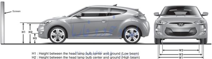
H3: Height between the fog lamp bulb center and ground
