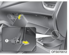
2. Loosen the screws (1) and then remove the glove box inner panel.
