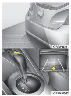
The rearview camera will activate when the back-up light is ON with the ignition switch ON and the shift lever in the R (Reverse) position.
