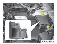
Engine compartment fuse panel
