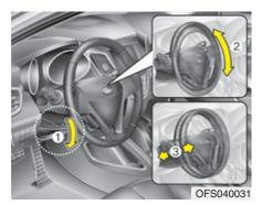
To change the steering wheel angle, pull down the lock release lever (1), adjust the steering wheel to the desired angle (2) and height (3), then pull up the lock-release lever to lock the steering wheel in place. Be sure to adjust the steering wheel to the desired position before driving.
