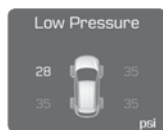
Low Tire Pressure Monitor with Location Indicator ( Shown on the LCD display )
