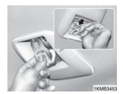
3. Insert the tongue plate (A) into the hole on the belt assembly cover.
