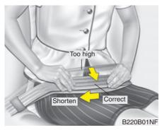
With a 2-point static type seat belt, the length must be adjusted manually so it fits snugly around your body. Fasten the belt and pull on the loose end to tighten. The belt should be placed as low as possible on your hips, not on your waist. If the belt is too high, it could increase the possibility of injury in an accident.
