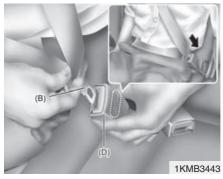
3. Pull the tongue plate (B) and insert the tongue plate (B) into the open end of the buckle (D) until an audible "click" is heard, indicating the latch is locked. Make sure the belt is not twisted.
