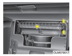
3. Remove the climate control air filter case while pressing the lock on the right of the cover.
