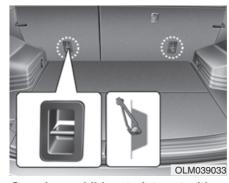
Securing a child restraint seat with "Tether Anchor" system (if equipped) Child restraint hook holders are located on the back of the rear seats.
