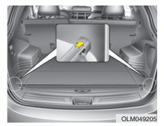
When not in use, place the cargo security screen on the lower portion of the cargo area. (if equipped)
