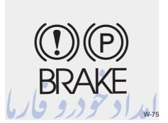
Check the brake warning light by turning the ignition switch ON (do not start the engine). This light will be illuminated when the parking brake is applied with the ignition switch in the START or ON position.
