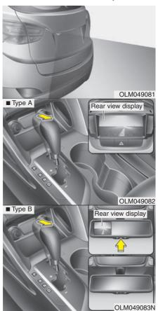
The rearview camera will activate when the back-up light is ON with the ignition switch ON and the shift lever in the R (Reverse) position.
