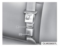
2. To retract the rear center seatbelt, insert the buckle into the web release hole (C). Pull up on the seat belt web (A) and allow the webbing to retract automatically.
