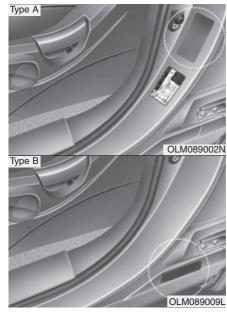
The vehicle certification label attached on the driver's (or front passenger's) side center pillar gives the vehicle identification number (VIN).
