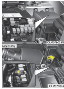
Engine compartment panel fuse replacement
