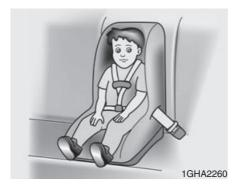
Installing a child restraint system with a lap belt (on the center rear seat) (if equipped) - Except Europe
