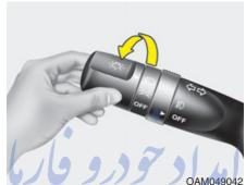
Headlight position ( (D) When the light switch is in the headlight position the head, tail, position, license and instrument panel lights are ON.
