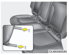
Both rear outboard seats are equipped with a pair of ISOFIX anchorages as well as a corresponding top tether anchorage on the back side of the back rest. The ISOFIX anchorages are located between seat cushion and back rest, marked with the ISOFIX icon.
