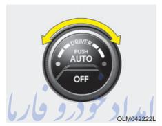
2. Set the desired temperature by turning the temperature control knob.
