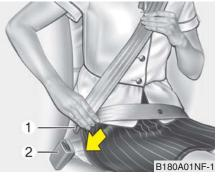
Seat belt - Driver's 3-point system with emergency locking retractor
