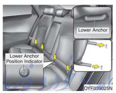
Child restraint symbols are located on the left and right rear seat backs to indicate the position of the lower anchors for child restraints. المناف روزي:
