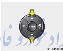
2. Set the temperature button to the desired temperature.
