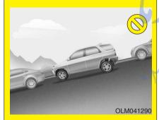
When the smart parking assist system is operated in slope road, driver needs to apply to accelerator and brake pedal by himself. If driver is unfamiliar with controlling the pedal, the crash accident may occur.
