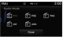
If [Pop-up Mode] is turned on within SETUP | [Display], then pressing the RADIO key will display the Radio Popup Mode screen.
