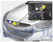
2. Go to the front of the vehicle, raise the bonnet slightly, pull the secondary latch (1) inside of the bonnet centre and lift the bonnet (2).
