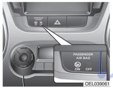
Passenger's front air bag ON indicator (if equipped)
