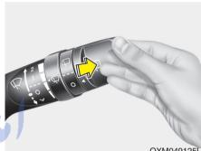
Push the lever away from you to spray rear washer fluid and to run the rear wipers 1~3 cycles. The spray and wiper operation will continue until you release the lever. (if equipped)
