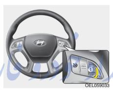
3. Move the lever (1) down (to SET-), and release it at the desired speed. The SET indicator light in the instrument cluster will illuminate. Release the accelerator pedal. The desired speed will automatically be maintained.
