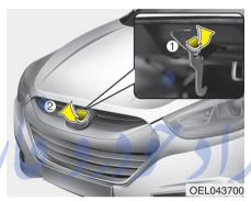
2. Go to the front of the vehicle, raise the hood slightly, pull the secondary latch (1) inside of the hood center and lift
