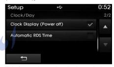
This feature is used to display a clock on the screen when the audio system is turned off.
