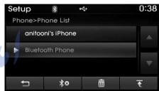
From the paired phone list, select the currently connected device and press the \*⊗ button.
