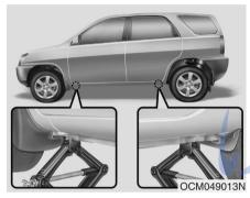
7. Place the jack at the front or rear jacking position closest to the tyre you are changing. Place the jack at the designated locations under the frame. The jacking positions are plates welded to the frame with two tabs and a raised dot to index with the jack.
