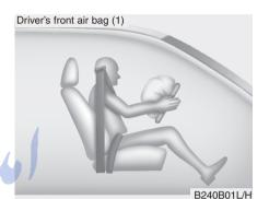
The front air bag modules are located both in the centre of the steering wheel and in the front passenger's panel above the glove box. When the SRSCM detects a sufficiently severe impact to the front of the vehicle, it will automatically deploy the front air bags.
