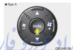
Operate the driver side temperature control to adjust the driver side temperature. Operate the passenger side temperature control to adjust the passenger side temperature.
