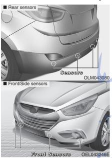
This is the parking assist system to warn the driver of object which are detected by front, rear and side sensors with range of distance of sensors operation as warning sound or indicator (LCD) when the vehicle is moved back or forward. This system is a supplemental system and it is not intended to nor does it replace the need for extreme care and attention of the driver.
