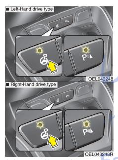
During operating system, warning sound is operated when objects are detected. To turn off this system, push the button of system choice over 2 seconds. After engine is off, if engine is turned on, this system is on position of turning off. If needed, push this button.
