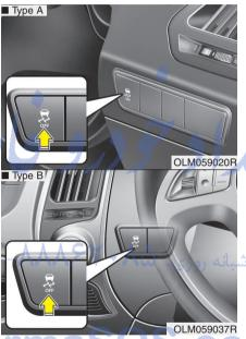
Electronic stability control (ESC) (if equipped)
