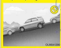
When the smart parking assist system is operated in slope road, driver needs to apply to accelerator and brake pedal by himself. If driver is unfamiliar with controlling the pedal, the crash accident may occur.
