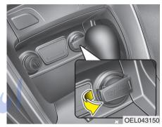
Connect between compressor and the vehicle power outlet using the cable and connectors.
