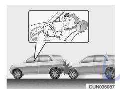
Air bags are not designed to inflate in rear collisions, because occupants are moved backward by the force of the impact. In this case, inflated air bags would not be able to provide any additional benefit.
