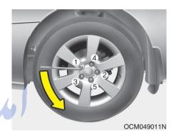
6. Loosen the wheel lug nuts counterclockwise one turn each, but do not remove any nut until the tyre has been raised off the ground.
