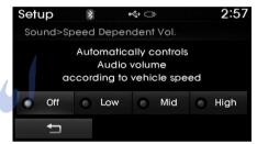
The volume level is controlled automatically according to the vehicle speed. SDVC can be set by selecting from Off/Low/Mid/High.
