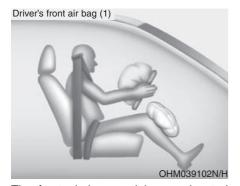
The front air bag modules are located both in the centre of the steering wheel, in the front passenger's panel above the glove box and/or in the driver's side knee bolster. When the SRSCM detects a sufficiently severe impact to the front of the vehicle, it will automatically deploy the front air bags.
