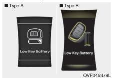
If the engine start/stop button changes to the OFF position when the smart key in the vehicle discharges, the warning illuminates on the LCD display for about 10 seconds. Also, the warning chime sounds once.
