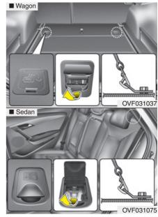
Securing a child restraint seat with "Tether Anchor" system (if equipped) Child restraint hook holders are located on the floor behind the rear seats (wagon) or the shelf behind the rear seats (sedan).
