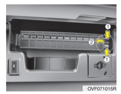
3. Remove the climate control air filter case whilst pressing the lock on the right side of the cover.
