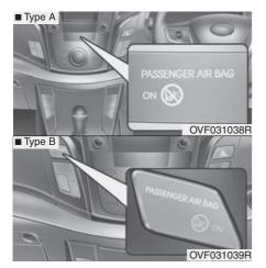
Passenger's front air bag ON indicator (if equipped)
