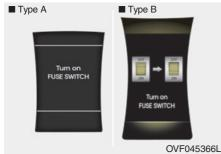
The notice appears to inform the driver to turn on the fuse switch in the instrument panel under the steering wheel.
