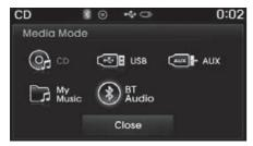
Turn the TUNE knob to move the focus. Press the knob to select.
