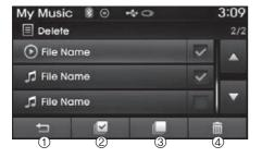
Press the button or individually select the files you want to delete. Once files are selected, the button and buttons will be enabled.
