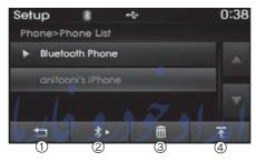
This feature is used to view mobile phones that have been paired with the audio system. Upon selecting a paired phone, the setup menu is displayed.
