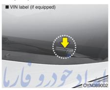
The VIN is also on a plate attached to the top of the dashboard. The number on the plate can easily be seen through the windscreen from the outside.
