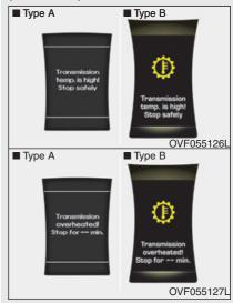
Under certain conditions such as repeated launch on steep grades, the clutch in the transmission could overheat. When the clutch is overheated, the safe protection mode engages. If the safe protection mode engages, the gear position indicator on the cluster blinks with a chime sound.
