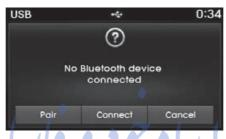
• If Bluetooth® Wireless Technology devices are paired but none are currently connected, pressing the key or the key or the steering remote controller displays the following screen. Press the [Pair] button to pair a new device or press the [Connect] to connect a previously pair device.
