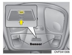
Intrusion/Tilt sensor ON/OFF condition
