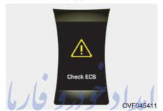
This warning message illuminates if there is a malfunction with the Electronic Control Suspension (ECS) system. We recommend that the vehicle be inspected by a HYUNDAI authorised repairer.
