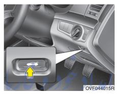
• To open the boot from inside the vehicle, press the boot lid release switch. Once the boot is opened and then closed, the boot locks automatically.
