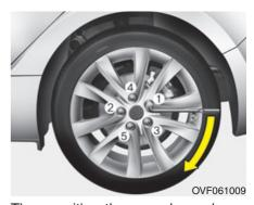
Then position the wrench as shown in the drawing and tighten the wheel nuts. Be sure the socket is seated completely over the nut. Do not stand on the wrench handle or use an extension pipe over the wrench handle. Go around the wheel tightening every nut following the numerical sequence shown in the image until they are all tight. Then double-check each nut for tightness. After changing wheels, we recommend that the system be checked by an authorised HYUNDAI repairer.
