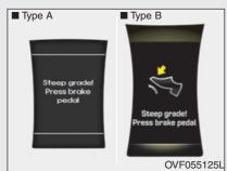
To hold the vehicle on a hill use the foot brake or the parking brake. If the vehicle is held by applying the accelerator pedal on a hill the clutch and transmission will be overheated resulting in damage.
