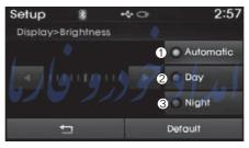
Use the buttons to adjust the screen brightness or set the Brightness on Automatic, Day, or Night mode.
