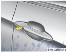
Carrying the smart key, you may lock and unlock the vehicle doors and boot.
