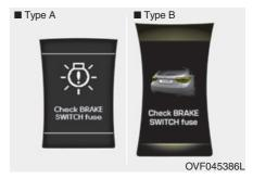
When the stop lamp fuse is disconnected, the warning illuminates for 10 seconds on the LCD display.
