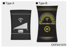
The illumination intensity of the instrument panel is shown when adjusting it with the illumination control switch.
