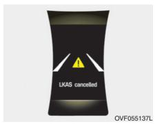
If the driver still does not have one's hand on the steering wheel after several seconds, the system will be automatically cancelled.
