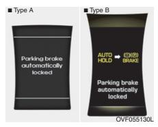
If the EPB is applied whilst Auto Hold is activated because of ESC(Electronic Stability Control) signal, a warning will sound and a message will appear.
