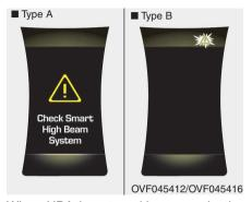
When HBA is not working properly, the warning message will come on for a few second. After the message disappears, the master warning light will illuminate. We recommend that the system be checked by an authorized HYUNDAI dealer.
