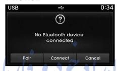
of Bluetooth® Wireless Technology devices are paired but none are currently connected, pressing the key or the key or the steering remote controller displays the following screen. Press the [Pair] button to pair a new device or press the [Connect] to connect a previously pair device.
