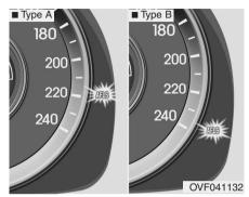
If the AFLS malfunction indicator comes on, the AFLS is not working properly. Drive to the nearest safe location and restart the engine. If the indicator continuously remains on, we recommend that the system be checked by an authorized HYUNDAI dealer.
