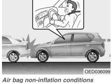
In certain low-speed collisions the air bags may not deploy. The air bags are designed not to deploy in such cases because they may not provide benefits beyond the protection of the seat belts in such collisions.
