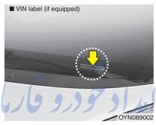
The VIN is also on a plate attached to the top of the dashboard. The number on the plate can easily be seen through the windshield from outside. تلفن شباله روزي:
