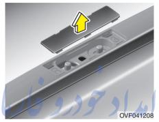
After using the roof carrier, install the cover back on the roof in the reverse order.
