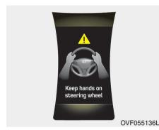
If the driver takes one's hands off the steering wheel while the LKAS is activated, the system will warn the driver after several seconds with a visual and audible warning.
