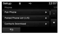
Bluetooth® Wireless Technology devices can be paired with the audio system. For more information, refer to the "Pairing through Phone Setup" section within Bluetooth® Wireless Technology.
