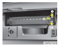
Remove the climate control air filter case while pressing the lock on the right side of the cover.
