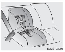
Installing a child restraint system by lap/shoulder belt
