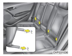
Both rear outboard seats are equipped with a pair of ISOFIX anchorages as well as a corresponding top tether anchorage on the floor behind the rear seats (wagon) or the shelf behind the rear seats (sedan). The ISOFIX anchorages are located between seat cushion and backrest, marked with the ISOFIX icon. For installation, CRS ISOFIX connecters have to engage with the vehicles ISOFIX anchorages (listen for a CLICK, check potential visual indicators on the CRS and cross-check by pulling).
