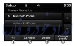
This feature is used to view mobile phones that have been paired with the audio system. Upon selecting a paired phone, the setup menu is displayed. For more information, refer to the "Setting
