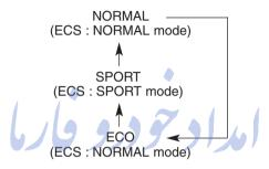
When the DRIVE mode changes, the ECS mode changes simultaneously. (Vehicles equipped with ECS)
