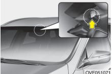
The Lane Keeping Assist System detects lane markers on the road, and assists the driver's steering to help keep the vehicle between lanes. When the system detects the vehicle straying from its lane, it alerts the driver with a visual and audible warning, while applying a slight counter-steering torque, trying to prevent the vehicle from moving out of its lane.
