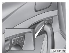
A driver position memory system is provided to store and recall the driver seat position with a simple button operation. By saving the desired position into the system memory, different drivers can reposition the driver seat based upon their driving preference. If the battery is disconnected, the position memory will be erased and the driving position should be restored in the system.
