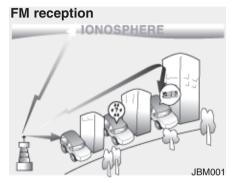
AM and FM radio signals are broadcast from transmitter towers located around your city. They are intercepted by the radio antenna on your vehicle. This signal is then received by the radio and sent to your vehicle speakers.
