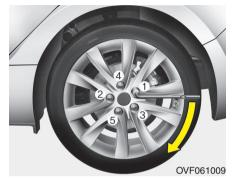
Then position the wrench as shown in the drawing and tighten the wheel nuts. Be sure the socket is seated completely over the nut. Do not stand on the wrench handle or use an extension pipe over the wrench handle. Go around the wheel tightening every nut following the numerical sequence shown in the image until they are all tight. Then double-check each nut for tightness. After changing wheels, we recommend that the system be checked by an authorized HYUNDAI dealer
