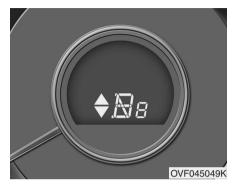
Dual Clutch Transmission Shift Indicator (if equipped)
