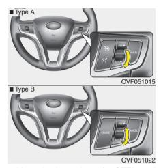
Move the lever down (to SET-), and release it at the desired speed. The cruise set indicator light will illuminate. Release the accelerator pedal at the same time. The desired speed will automatically be maintained.
