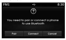
If Bluetooth® Wireless Technology devices are paired but none are currently connected, pressing the PHONE key or the key on the steering remote controller displays the following screen. Press the [Pair] button to pair a new device or press the [Connect] to connect a previously pair device.
