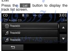
Turn the OTUNE knob left/right to search for tracks. Once the desired track is displayed, press the knob to select and play.
