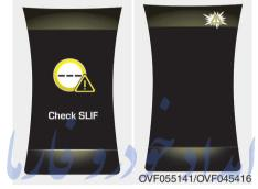
When SLIF is not working properly, the warning message will come on for a few second. After the message disappears, the master warning light will illuminate. We recommend that the system be checked by an authorized HYUNDAI dealer
