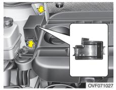
Engine compartment sub fuse panel (Diesel Engine)
