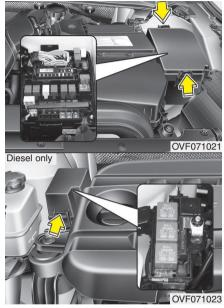
Engine compartment panel fuse replacement
