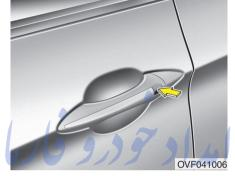
Carrying the smart key, you may lock and unlock the vehicle doors and tailgate.
