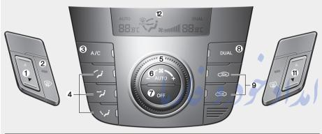
■ Type B (Vehicle equipped with AVN system)
