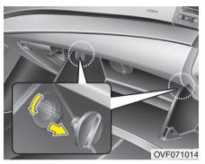
2. With the glove box open, remove the stoppers on both sides.
