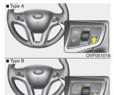
Fach of these actions will cancel cruise control operation (the cruise set indicator light will go off), but it will not turn the system off. If you wish to resume cruise control operation, move up the lever (to RES+) located on your steering wheel. You will return to your previously preset speed.
