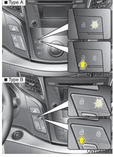
With central door lock/unlock switch It is operated by pressing the door lock/unlock switch.
