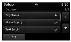
This feature is used to display the Mode Pop-up screen when entering radio and media modes.
