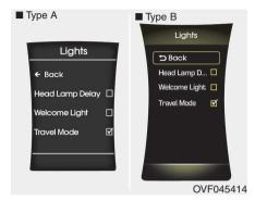
Check "Travel Mode" by pressing the move button (▼) and select button (◄) on the steering wheel.
