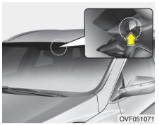
The system displays the information of speed limit and no passing restriction to the driver in both the instrument cluster and navigation screen. SLIF detects traffic signs with camera system attached behind the top of the windscreen.
