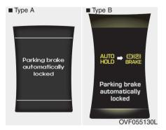
If the EPB is applied while Auto Hold is activated because of ESC (Electronic Stability Control) signal, a warning will sound and a message will appear.
