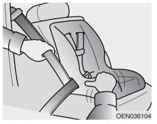
Buckle the seat belt and allow the seat belt to take up any slack. After installation of the child restraint system, try to move it in all directions to be sure the child restraint system is securely installed.
