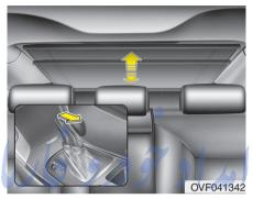
The rear curtain will fold automatically when you shift the shift lever into R (Reverse) and unfold automatically when you shift the shift lever from R (Reverse) into P (Park).
