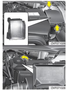
Engine compartment main fuse panel
