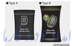
If the smart key is not in the vehicle or is not detected and you press the engine start/stop button, the warning illuminates on the LCD display for 10 seconds. Also,
