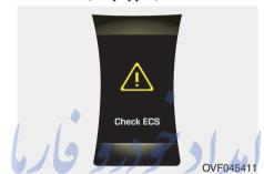
This warning message illuminates if there is a malfunction with the Electronic Control Suspension (ECS) system. We recommend that the vehicle be inspected by an authorized HYUNDAI dealer.
