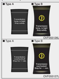
Under certain conditions such as repeated launch on steep grades, the clutch in the transmission could overheat. When the clutch is overheated, the safe protection mode engages. If the safe protection mode engages, the gear position indicator on the cluster blinks with a chime sound.
