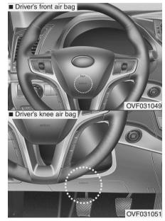
Driver's and passenger's front air bag (if equipped)
