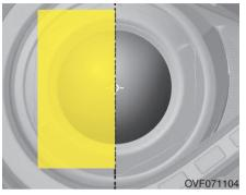
Left-hand drive country: Attach an adhesive tape on the left side of both low beams.
