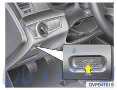
To open the trunk from inside the vehicle, press the trunk lid release switch.
