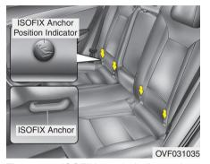
There are ISOFIX symbols located on the lower portion of each side of the rear seatbacks. These symbols indicate the position of the lower anchors for child restraints so equipped.
