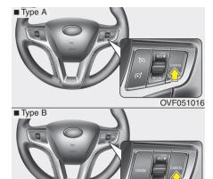
Fach of these actions will cancel cruise control operation (the cruise set indicator light will go off), but it will not turn the system off. If you wish to resume cruise control operation, move up the lever (to RES+) located on your steering wheel. You will return to your previously preset speed.
