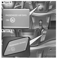
Passenger's front air bag ON indicator (if equipped)
