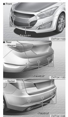
The parking assist system assists the driver during movement of the vehicle by chiming if any object is sensed within the distance of 60 cm (24 in.) in front and 100 cm (39 in.) behind the vehicle. This system is a supplemental system and it is not intended to nor does it replace the need for extreme care and attention of the driver.
