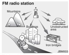
FM broadcasts are transmitted at high frequencies and do not bend to follow the earth's surface. Because of this, FM broadcasts generally begin to fade at short distances from the station.
