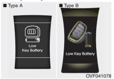
If the engine start/stop button changes to the OFF position when the smart key in the vehicle discharges, the warning illuminates on the LCD display for about 10 seconds. Also, the warning chime sounds once.
