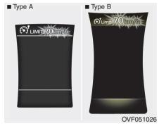
To drive over the preset speed limit you must depress hard on the accelerator pedal (more than approximately 80%) until the kick down mechanism works with a clicking noise. Then the set speed limit will blink and chime will sound until you return the vehicle speed within the speed limit.
