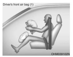
The front air bag modules are located both in the center of the steering wheel, in the front passenger's panel above the glove box and/or in the driver's side knee bolster. When the SRSCM detects a sufficiently severe impact to the front of the vehicle, it will automatically deploy the front air bags.
