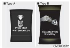
If you press the engine start/stop button while the warning "Key is not detected" illuminates the warning "Press the start button with smart key" illuminates for 10 seconds on the LCD display. Also, the immobilizer indicator blinks for 10 seconds.
