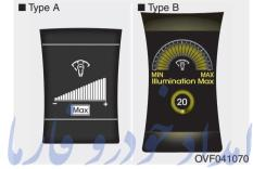
The illumination intensity of the instrument panel is shown when adjusting it with the illumination control switch.
