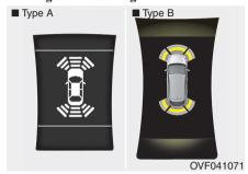
Displays the area an obstacle is detected while moving forward or rearward. For more details, refer to "Parking assist system" in section 4.
