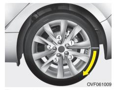
Then position the wrench as shown in the drawing and tighten the wheel nuts. Be sure the socket is seated completely over the nut. Do not stand on the wrench handle or use an extension pipe over the wrench handle. Go around the wheel tightening every nut following the numerical sequence shown in the image until they are all tight. Then double-check each nut for tightness. After changing have authorized wheels. an HYUNDAI dealer tighten the wheel nuts to their proper torque as soon as possible.
