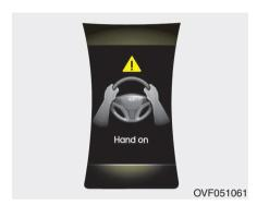
If the driver takes one's hands off the steering wheel while the LKAS is activated, the system will warn the driver after several seconds with a visual and audible warning.
