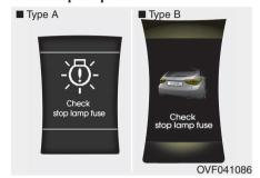
When the stop lamp fuse is disconnected, the warning illuminates for 10 seconds on the LCD display.
