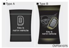
If the smart key is not in the vehicle and if any door is opened or closed with the engine start/stop button in the ACC, ON, or START position, the warning illuminates on the LCD display. Also, the chime sounds for 5 seconds when the smart key is not in the vehicle and the door is closed.
