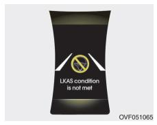
A message will appear on the LCD display if the condition to activate the LKAS is not satisfied. Also, an audible warning will be heard. The warning will disappear when the conditions are met.
