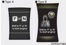
If you try to start the engine with the shift lever not in the P(Park) or N(Neutral) position, the warning illuminates for about 10 seconds on the LCD display.
