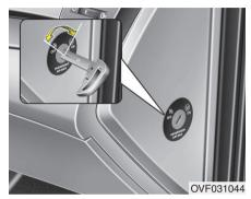
Passenger's front air bag ON/OFF switch (if equipped)
