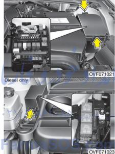
Engine compartment panel fuse replacement
