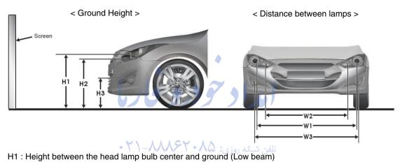
H2: Height between the head lamp bulb center and ground (High beam)
