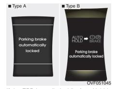
If the EPB is applied while Auto Hold is activated because of ESP(Electronic Stability Program) signal, a warning will sound and a message will appear.
