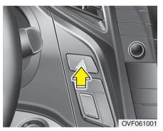
The hazard warning flasher should be used whenever you find it necessary to stop the car in a hazardous location. When you must make such an emergency stop, always pull off the road as far as possible.
