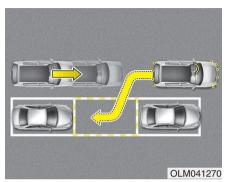
The Smart Parking Assist System helps drivers park their vehicle by using sensors to measure parallel parking spaces, control the steering wheel to semi-automatically park the car and provide instruction on the LCD display to help through parking.
