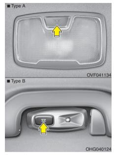
**Room lamp**Press the button to turn the light on or off.
