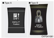
If you try to turn off the engine without the shift lever in the P (Park) position, the engine start/stop button will turn to the ACC position. If the button is pressed once more it will turn to the ON position. The warning illuminates on the LCD display for about 10 seconds to indicate that you should press the engine start/stop button with the shift lever in the P (Park) position to turn off the engine.
