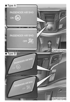
To deactivate or reactivate the passenger's front air bag:
