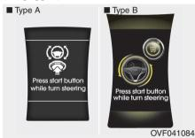
If the steering wheel does not unlock normally when the engine start/stop button is pressed, the warning illuminates for 10 seconds on the LCD display. Also, the warning chime sounds once and the engine start/stop button light blinks for 10 seconds.
