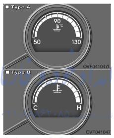
Engine coolant temperature gauge
