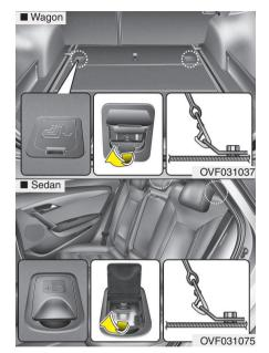
Securing a child restraint seat with "Tether Anchor" system (if equipped) Child restraint hook holders are located on the floor behind the rear seats (wagon) or the shelf behind the rear seats (sedan).
