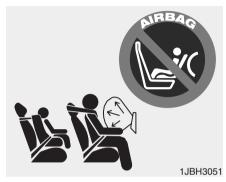
Installing a child restraint on a front passenger's seat is forbidden when the air bag is active
