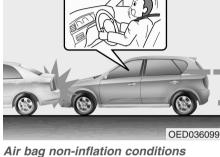
In certain low-speed collisions the air bags may not deploy. The air bags are designed not to deploy in such cases because they may not provide benefits beyond the protection of the seat belts in such collisions.
