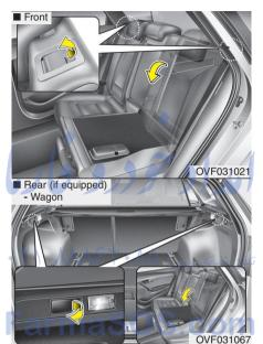
Pull on the seatback folding lever, then fold the seat toward the front of the vehicle.
