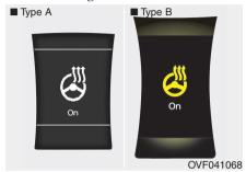
The indicator will appear when the heated steering wheel is turned on.
