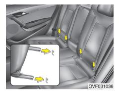
Both rear outboard seats are equipped with a pair of ISOFIX anchorages as well as a corresponding top tether anchorage on the floor behind the rear seats (wagon) or the shelf behind the rear seats (sedan). The ISOFIX anchorages are located between seat cushion and backrest, marked with the ISOFIX icon. For installation, CRS ISOFIX connecters
