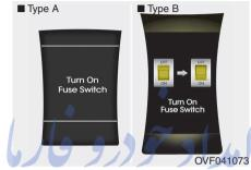
The notice appears to inform the driver to turn on the fuse switch in the instrument panel under the steering wheel.
