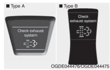
This warning message illuminates if the DPF system has a malfunction. At this time, DPF warning light also blinks.
