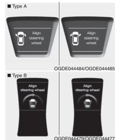
This warning message illuminates if you start the engine when the steering wheel is turned to more than 90 degrees to the left or right.
