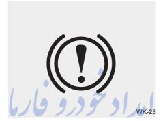
Check the brake warning light by turning the ignition switch ON (do not start the engine). This light will illuminate when the parking brake is applied with the ignition switch in the START or ON position.
