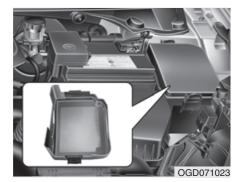
Engine compartment fuse panel
