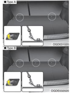
Securing a child restraint seat with "Tether Anchor" system (if equipped)
