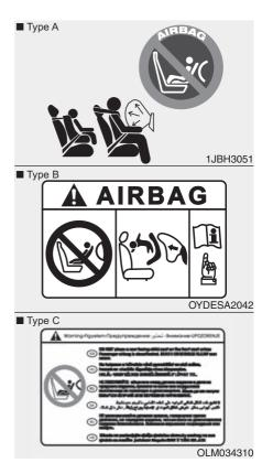
Do not install a child restraint on the front passenger's seat.
