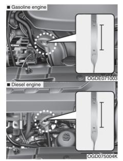
Checking the engine oil level
