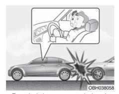
Frontal air bags are not designed to inflate in rear collisions, because occupants are moved backward by the force of the impact. In this case, inflated air bags would not be able to provide any additional benefit.
