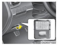
Fuse/relay panel description Inner fuse panel
