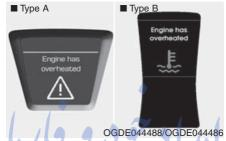
This warning message illuminates and warning sound activates 5 times when the engine coolant temperature is above 120°C (248°F). This means that the engine is overheated and may be damaged.
