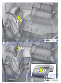
8. To use the rear seat, lift and push the seatback backward firmly until it clicks into place. Make sure the seatback is locked in place (red invisible).
