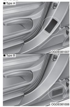
The vehicle certification label attached on the driver's (or front passenger's) side center pillar gives the vehicle identification number (VIN).
