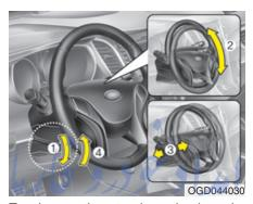
To change the steering wheel angle, push down the lock release lever (1), adjust the steering wheel to the desired angle (2) and height (3), then pull up the lock-release lever to lock the steering wheel in place (4). Be sure to adjust the steering wheel to the desired position before driving.
