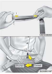
With a 2-point static type seat belt, the length must be adjusted manually so it fits snugly around your body. Fasten the belt and pull on the loose end to tighten. The belt should be placed as low as possible on your hips, not on your waist. If the belt is too high, it could increase the possibility of your being injured in an accident.
