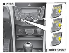
The seat warmer is provided to warm the front seats during cold weather. With the ignition switch in the ON position, push either of the switches to warm the driver's seat or the front passenger's seat.
