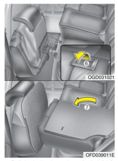
6. Pull the lock release lever (red visible).7. Fold the rear seatback forward and
