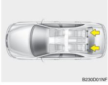
Securing a child restraint system with "ISOFIX" system and "Tether Anchorage" system (if equipped)
