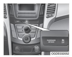
Passenger's front air bag OFF indicator (if equipped)
