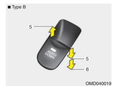
Type B - Auto down window (if equipped) Pressing the power window switch momentarily to the second detent position (6) completely lowers the window even when the switch is released. To stop the window at the desired position while the window is in operation, pull up the switch momentarily to the opposite direction of the window movement.
