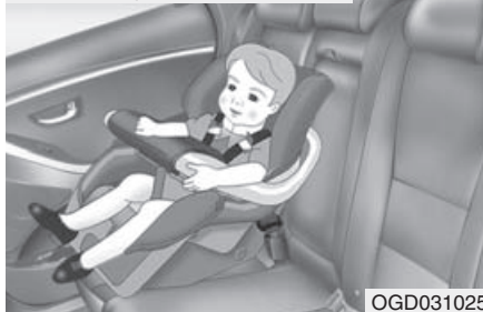
Forward-facing child restraint system
