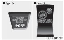
If the steering wheel does not unlock normally when the ENGINE START/STOP button is pressed, the warning illuminates for 10 seconds on the LCD display. Also, the warning chime sounds once and the ENGINE START/STOP button light blinks for 10 seconds.
