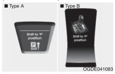
If you try to turn off the engine without the shift lever in the P (Park) position, the ENGINE START/STOP button will turn to the ACC position. If the button is pressed once more it will turn to the ON position. The warning illuminates on the LCD display for about 10 seconds to indicate that you should press the ENGINE START/STOP button with the shift lever in the P (Park) position to turn off the engine. Also, the warning chime sounds for about
