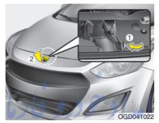
2. Go to the front of the vehicle, raise the hood slightly, push the secondary latch up (1) inside of the hood center and lift
