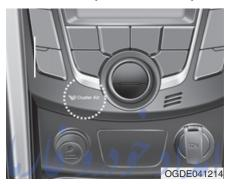
When the ignition switch is in the ON position, the clean air function turns on automatically.
