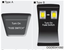
Turn on fuse switch (mode switch)
