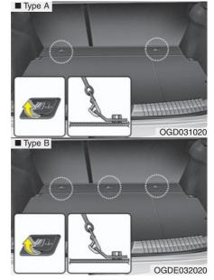
Securing a child restraint seat with "Tether Anchor" system (if equipped)
