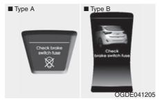
When the brake switch fuse is disconnected, the warning illuminates for 10 seconds on the LCD display.
