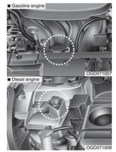
Check the condition and connections of all cooling system hoses and heater hoses. Replace any swollen or deteriorated hoses.
