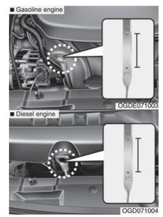
Checking the engine oil level
