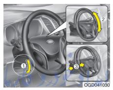
To change the steering wheel angle, push down the lock release lever (1), adjust the steering wheel to the desired angle (2) and height (3), then pull up the lock-release lever to lock the steering wheel in place. Be sure to adjust the steering wheel to the desired position before driving.
