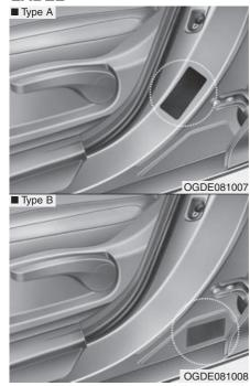
The vehicle certification label attached on the driver's (or front passenger's) side center pillar gives the vehicle identification number (VIN).
