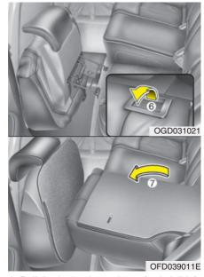
6. Pull the lock release lever (red visible).
