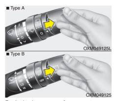
Push the lever away from you to spray rear washer fluid and to run the rear wipers 1~3 cycles. The spray and wiper operation will continue until you release the lever. (if equipped)
