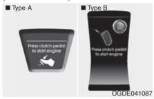
If the ENGINE START/STOP button turns to the ACC position twice by pressing the button repeatedly without depressing the clutch pedal, the warning illuminates on the LCD display for about 10 seconds to indicate that you should depress the clutch pedal to start the engine.
