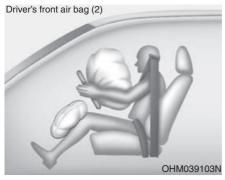
Upon deployment, tear seams molded directly into the pad covers will separate under pressure from the expansion of the air bags. Further opening of the covers then allows full inflation of the air bags.
