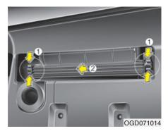
Remove the climate control air filter cover while pressing the lock on the both side of the cover.
