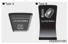
If the ENGINE START/STOP button turns to the OFF position when the smart key in the vehicle discharges, the warning illuminates on the LCD display for about 10 seconds. Also, the warning chime sounds once.
