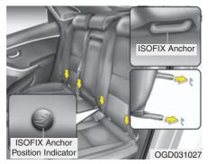
There are child restraint symbols located on the lower portion of each side of the rear seatbacks. These symbols indicate the position of the lower anchors for child restraints so equipped. Both rear outboard seats are equipped with a pair of ISOFIX anchorages as well as a corresponding top tether anchorage on the back side of the back rest. The ISOFIX anchorages are located between seat cushion and back rest, marked with the ISOFIX icon.
