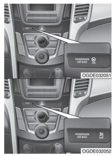
To deactivate or reactivate the passenger's front air bag:
