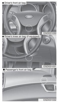
Driver's and passenger's front air bag (if equipped)
