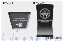
If the steering wheel does not lock normally when the ENGINE START/STOP button turns to the OFF position, the warning illuminates for 10 seconds on the LCD display. Also, the warning chime sounds for 3 seconds and the ENGINE START/STOP button light blinks for 10 seconds.
