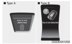
If the smart key is not in the vehicle or is not detected and you press the ENGINE START/ STOP button, the warning illuminates on the LCD display for 10 seconds. Also, the immobilizer indicator blinks for 10 seconds.
