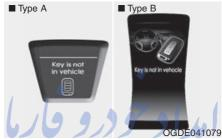
If the smart key is not in the vehicle and if any door is opened or closed with the ENGINE START/STOP button in the ACC, ON, or START position, the warning illuminates on the LCD display. Also, the chime sounds for 5 seconds when the smart key is not in the vehicle and the door is closed.
