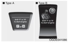
If you try to start the engine with the shift lever not in the P(Park) or N(Neutral) position, the warning illuminates for about 10 seconds on the LCD display. You can also start the engine with the shift lever in the N(Neutral) position, but for your safety start the engine with the shift lever in the P(Park) position.
