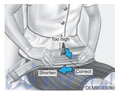
With a 2-point static type seat belt, the length must be adjusted manually so it fits snugly around your body. Fasten the belt and pull on the loose end to tighten. The belt should be placed as low as possible on your hips, not on your waist. If the belt is too high, it could increase the possibility of your being injured in an accident.
