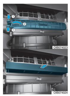
3. Remove the climate control air filter cover (2) by pushing or pressing the clip (1) on left side.
