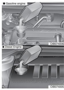
If it is near or at L (Low), add enough oil to bring the level to F (Full). **Do not overfill.**
