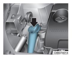
Check the fluid level in the washer fluid reservoir and add fluid if necessary. Plain water may be used if washer fluid is not available.
