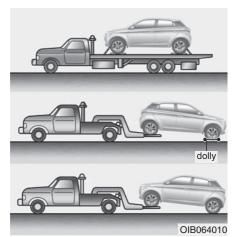
If emergency towing is necessary, we recommend having it done by an authorized HYUNDAI dealer or a commercial tow-truck service. Proper lifting and towing procedures are necessary to prevent damage to the vehicle. The use of wheel dollies or flatbed is recommended.
