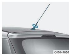
Your car uses a roof antenna to receive both AM and FM broadcast signals. This antenna is a removable type. To remove the antenna, turn it counterclockwise. To install the antenna, turn it clockwise.
