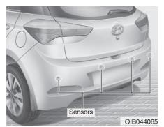
The Rear Parking Assist System aids the driver during reverse movement of the vehicle by chiming if any object is sensed within the distance of about 120 cm (47 in.) behind the vehicle. This is a supplemental system that senses objects within the range and location of the sensors, it cannot detect objects in other areas where sensors are not installed.
