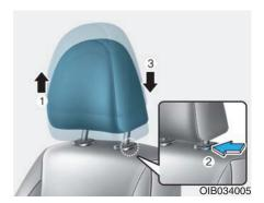
Adjusting the height up and down To raise the headrest, pull it up to the desired position (1). To lower the headrest, push and hold the release button (2) on the headrest support and lower the headrest to the desired position (3).
