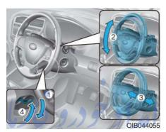
Pull down the lock-release lever (1) on the steering wheel column and adjust the steering wheel angle (2) and position (3). Move the steering wheel, so it points toward your chest, not toward your face. Make sure you can see the instrument panel warning lights and gauges.
