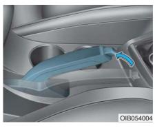
Always set the parking brake before leaving the vehicle, to apply:
