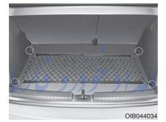
To keep items from shifting in the cargo area, you can use the 4 holders located in the cargo area (under the floor panel) to attach the luggage net. Make sure the luggage net is securely attached to the holders in the cargo area.
