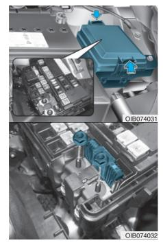
If the main fuse is blown, it must be removed as follows:
