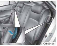
Insert the rear lap/shoulder belt plate into the holder on the side trim. It will prevent the lap/shoulder belt from interfering with the seatback when folding.
