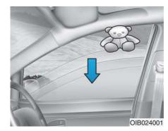
If a window senses any obstacle while it is closing automatically, it will stop and lower approximately 30 cm (12 in.) to allow the object to be cleared.
