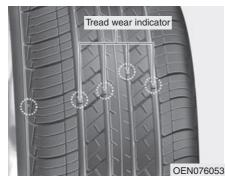
If the tire is worn evenly, a tread wear indicator will appear as a solid band across the tread. This shows there is less than 1.6 mm (1/16 inch) of tread left on the tire. Replace the tire when this happens.
