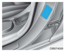
The vehicle certification label attached on the driver's (or front passenger's) side center pillar gives the vehicle identification number (VIN).
