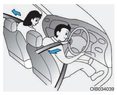
Your vehicle is equipped with driver's and front passenger's pre-tensioner seat belts. The purpose of the pre-tensioner is to make sure that the seat belts fit tightly against the occupant's body in certain frontal collisions. The pre-tensioner seat belts may be activated in crashes where the frontal collision is severe enough.
