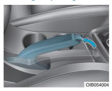
Check the stroke of the parking brake by counting the number of "clicks" heard while fully applying it from the released position. Also, the parking brake alone should securely hold the vehicle on a fairly steep grade. If the stroke is more or less than specified, we recommend that the system be inspected by an authorized HYUNDAI dealer.
