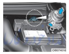
If you drive until you have no fuel left or if you replace the fuel filter, be sure to extract air from the fuel system as it makes it difficult to start the engine.
