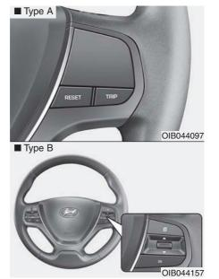
The trip computer is a microcomputer-controlled driver information system that displays information related to driving, when the ignition switch is in the ON position. All stored driving information (except odometer) resets if the battery is disconnected.
