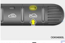
FRESH MODE ( ): The indicator light on the button is illuminated when the air intake control is in fresh mode.
