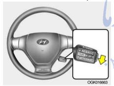
The vehicle will automatically resume the speed set prior to cancellation when you push the control switch upward to "RESUME (ACCEL)" position and release it to return providing the vehicle speed is above 25 mph (40 km/h).
