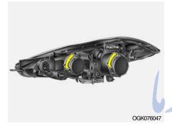
5. Turn the plastic cover counterclockwise and remove it.
