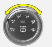
This is used to direct the flow of air. Air can be directed to the floor, dashboard outlets, or windscreen. Five symbols are used to represent Face, Bi-Level, Floor, Floor-Defrost and Defrost air position.
