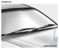
The wiper blades should be carefully inspected from time to time and cleaned to remove accumulations of road film or other debris. To clean the wiper blades and arms, use a clean sponge or cloth with a mild soap or detergent and water. If the wipers continue to streak or smear the glass, replace them with genuine Hyundai replacement.
