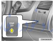
The Electronic Stability Program (ESP) system is designed to stabilise the vehicle during cornering manoeuvres. ESP checks where you are steering and where the vehicle is actually going. ESP applies the brakes at individual wheels and intervenes in the engine management system to stabilise the vehicle.
