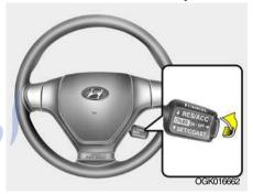
To disengage the cruise control system, Pull the control switch toward the steering wheel to "CANCEL" position. Additionally, the following actions will disengage the system:
