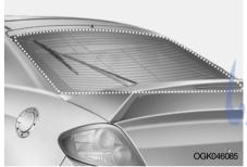
When the radio power switch is turned on whilst the ignition key is in either the "ON" or "ACC" position, your car will receive both AM and FM broadcast signals through the antenna in the rear window glass.
