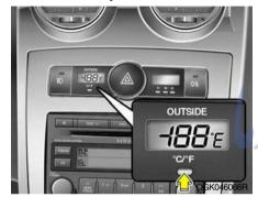
Press the button, the display show that the unit of outside temperature is adjusted to centigrade or fahrenheit (°C  $\rightarrow$  °F or °F  $\rightarrow$  °C).
