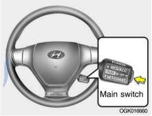
The cruise control system provides a constant speed hold function which may be determined at will. The system is most suited to use during dual carriageway/motorway driving where constant speed motoring at speeds in excess of 25 mph (40 km/h) may be undertaken.
