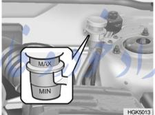
The clutch fluid level in the master cylinder should be checked when performing other under hood services. The system should be checked for leakage at the same time. Check to make certain that the clutch fluid level is always between the "MAX" and "MIN" level markings on the fluid reservoir. Fill as required. Fluid loss indicates a leak in the clutch system which should be inspected and repaired immediately. Consult your Hyundai dealer.
