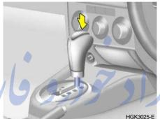
The highly efficient Hyundai automatic transaxle has four forward speeds and one reverse speed. The individual speeds are selected automatically, depending on the position of the selector lever. The selector lever has 2 gates; the main gate and the manual gate.
