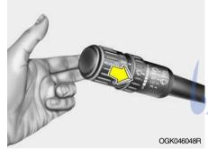
To use the windscreen washer, pull the wiper/washer lever toward the steering wheel. When the washers are operated, the wipers automatically make two passes across the windscreen. The washer continues to operate until the lever is released.
