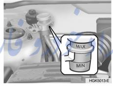
The clutch fluid level in the master cylinder should be checked when performing other under bonnet checks. The system should be checked for leakage at the same time.
