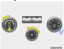
o Adjust the fan control to the desired speed. For greater cooling, turn the fan control to one of the higher speeds or temporarily select the recirculate ( position on the air intake control switch.
