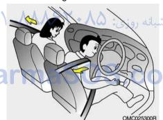
When the vehicle stops suddenly, or if the occupant tries to lean forward too quickly, the seat belt retractor will lock into position. In certain frontal collisions, the pre-tensioner will activate and pull the seat belt into tighter contact against the occupant's body.
