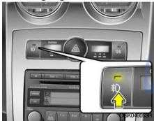
To turn on the rear fog lights, push the switch. They will light when the headlight switch is in the second position and the key is in the "ON" position.
