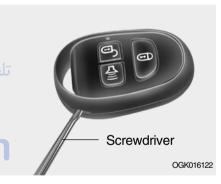
Carefully seperate the case with a blade screwdriver as shown in the illustration.
