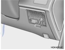
The fuse box containing the individual circuit fuses is located on the lower portion of the dashboard adjacent to the bonnet release. The fuse box cover is removed by pushing lightly and then releasing the lid. A fuse rating grid will be found on the reverse side of the cover. In the event of fuse failure, the fuse should be replaced with one of equivalent rating. A fuse removal tool is provided within the fuse box to facilitate replacement.
