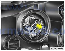
Disconnect the connector from the bulb base in the back of the headlight.
