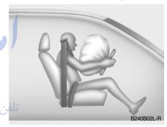
The airbag modules are located both in the centre of the steering wheel and in the front passenger's panel above the glove box. When the SRSCM detects a considerable impact to the front of the vehicle, it will automatically deploy the airbags.
