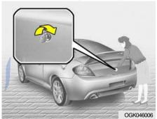
To open the hatchback door using the ignition key, insert the key into the lock barrel and turn clockwise to release the latch. The hatchback door compartment light will illuminate whenever the hatchback door is opened.
