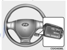
The steering wheel audio remote control switch is installed to promote safe driving.
