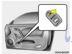
The hatchback door may be opened by pulling the lever to release the lock. The hatchback door should be closed by depressing the lid firmly until the latch engages. Ensure that hatchback door is securely latched before setting the vehicle in motion.
