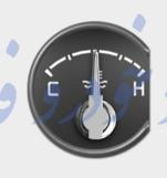
The needle on the engine coolant temperature gauge should stay in the normal range. If it moves across the dial to "H" (Hot), pull over and stop as soon as possible and turn off the engine. Then open the hood and, after the engine has cooled, check the coolant level and the water pump drive belt. If you suspect cooling system trouble, have your cooling system checked by a Hyundai dealer as soon as possible.
