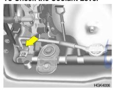
The coolant level can be seen on the side of the plastic coolant reservoir. The level of the coolant should be between the "L" and "F" lines on the reservoir when the engine is cool. If the level is below the "L" mark, add engine coolant to bring it up between "L" and "F". If the level is low, inspect for coolant leaks and recheck the fluid level frequently. If the level drops again, visit your Hyundai dealer for an inspection and diagnosis of the reason.
