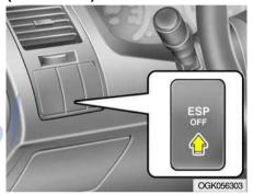
The Electronic Stability Program (ESP) system is designed to stabilize the vehicle during cornering manuevers. ESP checks where you are steering and where the vehicle is actually going. ESP applies the brakes at individual wheels and intervenes in the engine management system to stabilize the vehicle.
