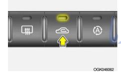
This is used to select fresh outside air or recirculate inside air automatically.
