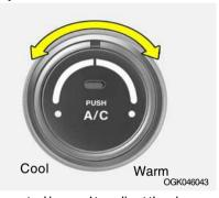
This control is used to adjust the degree of heating or cooling desired.
