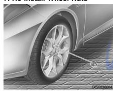
To reinstall the wheel, hold it on the studs, put the wheel nuts on the studs and tighten them finger tight. The nuts should be installed with their small diameter ends directed inward. Jiggle the tire to be sure it is completely seated, then tighten the nuts as much as possible with your fingers again.
