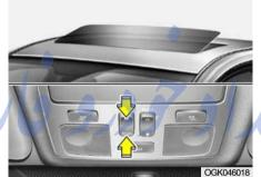
To use the auto tilt feature, press the UP button on the overhead console. The sunroof will tilt all the way open. To stop the sunroof tilting at any point, press any sunroof control button.
