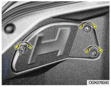
5. To remove the cover of the rear luggage trim, turn the knob by hand to the counterclockwise.
