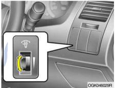
The level of illumination intensity of the instrument panel may be varied by turning the control shown. The instrument panel will be illuminated when the side light or headlights are in operation.
