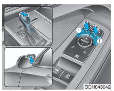
When you move the shift lever to the R (Reverse) position, the outside rearview mirror(s) will rotate downwards to aid with driving in reverse. The position of the outside rearview mirror switch (1) determines whether or not the mirrors will move:
