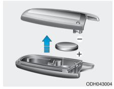
Battery Type: CR2032 To replace the battery:
