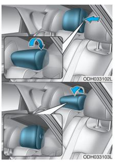
Folding the center headrest To fold the center headrest:
