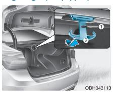
Pull the strap (1) to hang a bag on the hook (2). Fold the hook when not in use.
