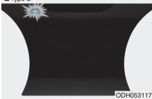
The LKAS failure indicator (yellow) will illuminate if the LKAS is not working properly. Have your vehicle checked by an authorized HYUNDAI dealer.
