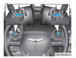
The paddle shifter is available when the shift lever is in the D (Drive) position or the sports mode. With the shift lever in the D position
