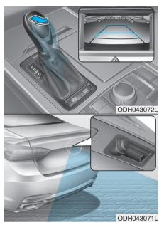
The Parking Guide System (PGS) will activate when the back-up light is ON with the Engine Start/Stop button ON and the shift lever in the R (Reverse) position.
