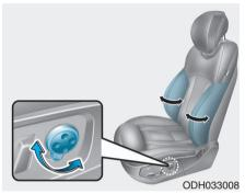
Seat bolster adjustment (for driver's seat, if equipped)
