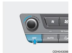
Push the OFF button of the front to turn off the air climate control system. However, you can still operate the mode and air intake buttons as long as the Engine Start/Stop button is in the ON position.
