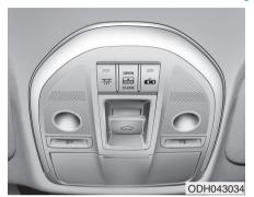
The Engine Start/Stop button must be in the ON position before you can open or close the sunroof.
