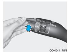
To turn on the high beam headlamp, push the lever away from you. The lever will return to its original position. The high beam indicator will light when the headlamp high beams are
