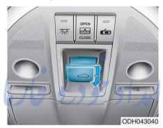
Whenever the vehicle battery is disconnected or discharged, or related fuse is blown, you must reset your sunroof system as follows:
