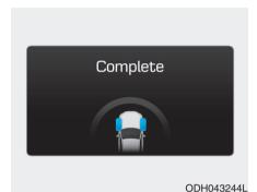
If the steering wheel aligning is completed after "Align steering wheel" warning message is displayed, this message is displayed for 2 seconds.
