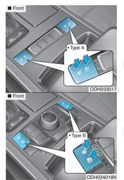
The seat warmers and coolers are provided to warm or cool the front seats by blowing air through small vent holes on the surface of the seat cushions and seatbacks.
