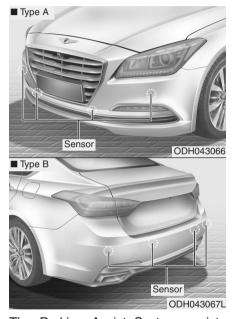
The Parking Assist System assists the driver during movement of the vehicle by chiming if any object is sensed within the distance of 39 inches (100 cm) in front and 47 inches (120 cm) behind the vehicle.
