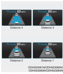
Your vehicle speed will slow down or speed up to maintain the selected distance.  If the vehicle ahead speeds up, your vehicle will travel at a steady cruising speed after accelerating to the set speed.
