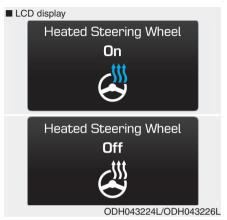
When the Engine Start/Stop button is in the ON position, press the heated steering wheel button to warm the steering wheel. The indicator on the button will illuminate and notify you on the LCD display.
