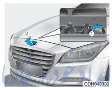
3. Raise the hood slightly, push the secondary latch up (1) inside of the hood center and lift the hood
