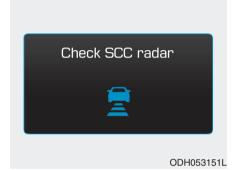
If the sensor or cover is dirty or obscured with foreign matter such as snow, the message will appear. Clean the sensor or cover by using a soft cloth.
