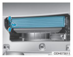
3. Remove the climate control air filter case by pulling out left sides of the cover.
