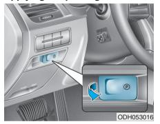
To apply the EPB (Electric Parking Brake):
