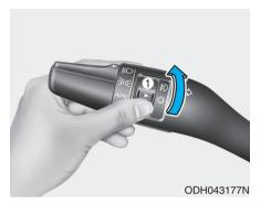
Use the switch next to the headlamp switch to turn the Fog Lights ON and OFF. The fog lamps will turn on when the fog lamp switch (1) is turned to the ON position after the headlamps are turned on.
