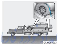
When towing the vehicle by flatbed equipment, secure wheels by using chocks and tie-down straps (or soft belts).
