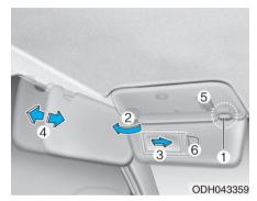
To use a sunvisor, pull it downward. To use a sunvisor for a side window, pull it downward, unsnap it from the bracket (1) and swing it to the side (2). To use the vanity mirror, pull down the sunvisor and slide the mirror cover (4). Adjust the sunvisor forward or backward (3) as needed. Use the ticket holder (5 and 6) to hold tickets.
