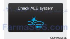
When the AEB system is turned off, the AEB warning light turns on. (Warning message does not come on.)
