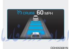
This mode displays the state of the Advanced Smart Cruise Control (ASCC) and Lane Keeping Assist System (LKAS).
