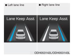
If all the conditions to activate LKAS is not satisfied, the system will convert to LDWS and warn the driver only when the driver crosses the lane lines.
