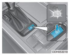
1. Press the [AUTO HOLD] switch. The AUTO HOLD indicator will illuminate white and the system will be in the standby position.
