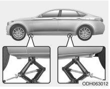
8. Place the jack at the designated jacking position under the frame closest to the tire you are changing. The jacking positions are plates welded to the frame with two tabs and a raised dot. Never jack any other position or part of the vehicle. It may damage to the side seal molding.
