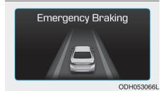
A warning message and chime will sound when you need to use the brake pedal or steering wheel due to a sudden stop or lack of distance with the vehicle ahead. The warning messages will vary according to the severity of the situation. Immediately reduce your speed to prevent a collision.
