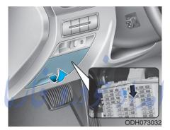
If you move the switch to the OFF position, some items such as audio and digital clock must be reset and the smart key may not work properly.
