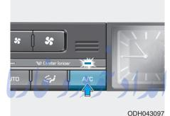
Push the A/C button to turn the air conditioning system on (indicator light will illuminate).
