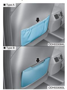
The seatback pocket is provided on the back of the front seatbacks.
