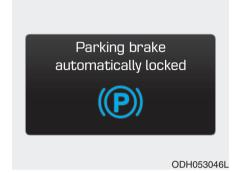
Parking brake automatically locked If the EPB is applied while Auto Hold is activated, a warning will sound and a message will appear.
