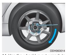
14. Use the wheel lug nut wrench to tighten the lug nuts in the order shown. Double-check each lug nut until they are tight. After changing tires, we recommend that an authorized HYUNDAI dealer tighten the lug nuts to their proper torque as soon as possible. The wheel lug nut should be tightened to 65~79 lb.ft (9~11 kg.m).
