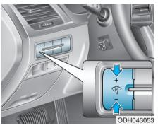
When the Engine Start Stop button is in the ON position, press the illumination control button to adjust the instrument panel illumination intensity and AVN monitor illumination intensity.
