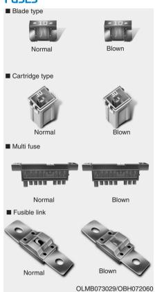
A vehicle's electrical system is protected from electrical overload damage by fuses.
