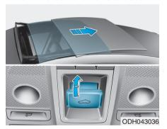
If you pull the sunroof control lever backward, the sunshade will slide all the way open then the sunroof class will slide all the way open. To stop the sunroof movement at any point, pull sunroot movement at any point, pull or push the sunroof control lever momentarily.
