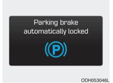
Parking brake automatically locked When the EPB is applied from Auto Hold, a warning will sound and a message will appear.
