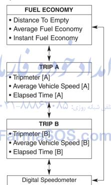
To change the trip mode, rotate the MOVE switch " $\blacktriangle$ ,  $\blacktriangledown$ " on the steering wheel.
