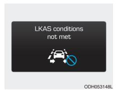
A message will appear on the LCD display if the condition to activate the LKAS is not satisfied. Also, there will be an acoustic warning. The warning will disappear when the conditions are met.
