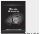
8. After using the EPB emergency release, a warning message will come on. You should operate the EPB switch for the vehicle to return to its normal condition. If the vehicle does not return to normal condition, take your vehicle to an authorized HYUNDAI dealer and have the system checked.
