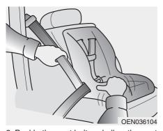
3. Buckle the seat belt and allow the seat belt to take up any slack. After installation of the child restraint system, try to move it in all directions to be sure the child restraint system is securely installed.
