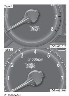
ECS (Electronic Controlled Suspension) Malfunction indicator
