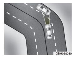
Your vehicle speed can be reduced due to a vehicle in the adjacent lane. Apply the accelerator pedal and select the appropriate set speed. Check to be sure that the road conditions permit safe operation of the smart cruise control.
