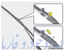
2. Open the cover of the blade. Press the clip behind the wiper arm and remove the blade assembly downward.
