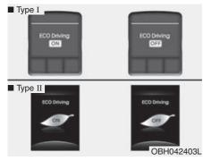
ECO Driving ON/OFF mode (if equipped) You can turn the ECO indicator on/off on the instrument cluster in this mode.
