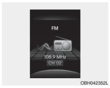
AV information (if equipped) This mode displays the state of the AV (RADIO, CD, USB, AUX etc.).
