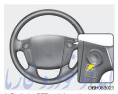
Push the SET- switch, and release it at the desired speed. The SET indicator light in the instrument cluster will illuminate. Release the accelerator pedal. The desired speed will automatically be maintained.
