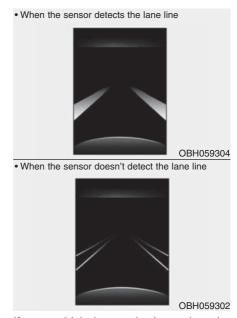
If your vehicle leaves the lane when the LDWS is operating and vehicle speed exceeds 60km/h, the warning operates as follows:
