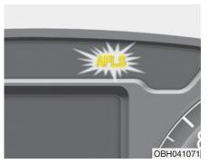
If the AFLS malfunction indicator comes on, the AFLS is not working properly. Drive to the nearest safe location and restart the engine. If the indicator continuously remains on, take your vehicle to an authorized HYUNDAI dealer and have the system checked.
