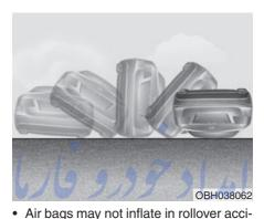
dents because air bag deployment would not provide protection to the occupants.
