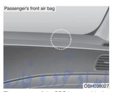
The purpose of the SRS is to provide the vehicle's driver and/or the front passenger with additional protection than that offered by the seat belt system alone in case of a frontal impact of sufficient severity.
