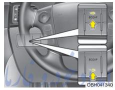
The ECO-P (pedal) indicator light will illuminate when the ECO-P button is pressed. If the fuel efficiency is low, the reactive force of intelligent accelerator pedal will be increased. It is allow to control over excess acceleration and you can drive fuel efficiently to help you improve fuel efficiency.
