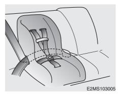
C030102AUN Installing a child restraint system by lap/shoulder belt
