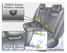
There is a child restraint symbol located on the lower portion of each side of the rear seatbacks. These symbols indicate the position of the lower anchors for child restraints so equipped.
