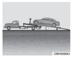
When you load the vehicle onto the tow truck, the loading angle(1) should be smaller than  $6^{\circ}$ .
