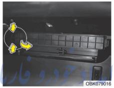
Remove the climate control air filter case pulling out both sides of the cover.
