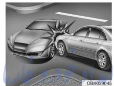
Front air bags may not inflate in side impact collisions, because occupants move to the direction of the collision, and thus in side impacts, frontal air bag deployment would not provide additional occupant protection.
