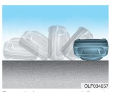
Front air bags may not inflate in rollover accidents because front air bag deployment would not provide additional occupant protection.
