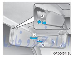
To use a sunvisor, pull it downward. To use a sunvisor for a side window, pull it downward, unsnap it from the bracket (1) and swing it to the side (2).
