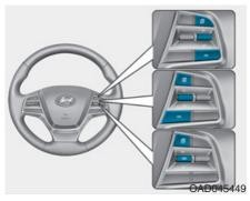
To change the trip mode, toggle the "▲, ▼" switch on the steering wheel.
