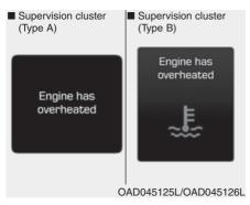
This warning message is displayed when the engine coolant temperature is above 120°C (248°F). This means that the engine is overheated and may be damaged.
