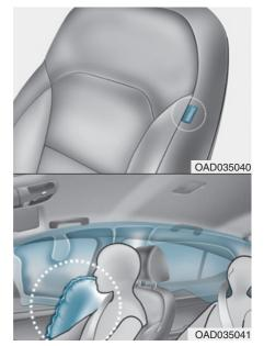
Your vehicle is equipped with a side air bag in each front seat. The purpose of the air bag is to provide the vehicle's driver and the front passenger with additional protection than that offered by the seat belt alone.
