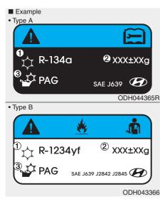
The actual Air Conditioning refrigerant label in the vehicle may differ from the illustration.
