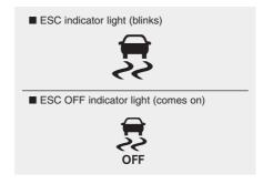
When the ignition switch is pressed to the ON position, the ESC indicator light illuminates, then goes off if the ESC system is operating normally.
