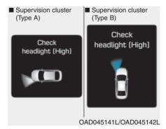
This warning message is displayed if the headlamps are not operating properly. The headlamp bulb may need to be replaced.
