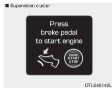
This warning message is displayed if the Engine Start/Stop button changes to the ACC position twice by pressing the button repeatedly without depressing the brake pedal.
