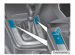
While the engine is running, push either of the switches to warm the driver's seat or front passenger's seat.
