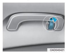
To hang items, pull the hanger down. These hangers are not designed to hold large or heavy items.
