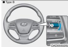
Push the toggle switch (1) down (SET-) and hold it. Your vehicle will gradually slow down. Release the toggle switch at the speed you want to maintain.
