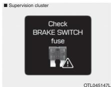
This warning message is displayed if the brake switch fuse is disconnected. You need to replace the fuse with a new one before starting the engine. If that is not possible, you can start the engine by pressing the Engine Start/Stop button for 10 seconds in the
