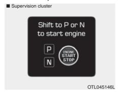
This warning message is displayed if you try to start the engine with the shift lever not in the P (Park) or N (Neutral) position.
