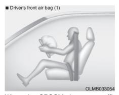
When the SRSCM detects a sufficiently severe impact to the front of the vehicle, it will automatically deploy the front air bags.
