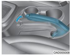
Always set the parking brake before leaving the vehicle, to apply: Firmly depress the brake pedal. Pull up the parking brake lever as far as possible.
