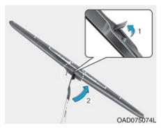
2. Lift up the wiper blade clip (1). Then lift up the wiper blade (2).
