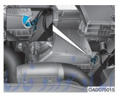
1. Loosen the air cleaner cover attaching clips and open the cover.
