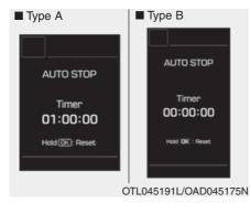
This mode displays the elapsed time of Auto stop for "Idle stop and go system".
