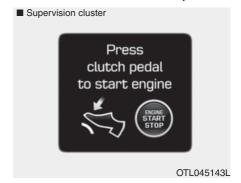
This warning message is displayed if the Engine Start/Stop button is in the ACC position twice by pressing the button repeatedly without depressing the clutch pedal.
