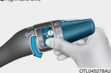
Vehicle without front fog lamp To turn on the rear fog lamp: Position the light switch in the headlamp position, and then turn the light switch (1) to the rear fog lamp position.
