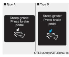
To hold the vehicle on a hill use the foot brake or the parking brake. If the vehicle is held by applying the accelerator pedal on a hill the clutch and transmission will be overheated resulting in damage.
