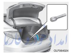
1. Open the trunk, and remove the towing hook from the tool case.
