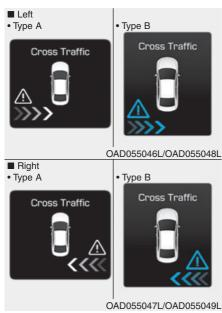
If the vehicle detected by the sensors approaches your vehicle, the warning chime will sound, the warning light on the outside rearview mirror will blink and a message will appear on the LCD display.
