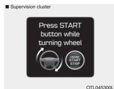
This warning message is displayed if the steering wheel does not unlock normally when the Engine Start/Stop button is pressed.
