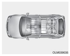
ISOFIX anchorages have been provided in the left and right outboard rear seating positions. Their locations are shown in the illustration. There are no ISOFIX anchorages provided for the center rear seating position.
