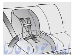
**Installing a Child Restraint System** with a lap/shoulder belt
