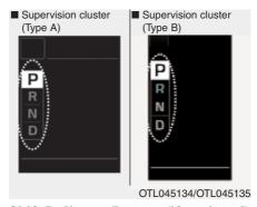
Shift Indicator Pop-up (if equipped) The pop-up that indicates the current gear position is displayed in the cluster for about 2 seconds when shifting into other positions (P/R/N/D).
