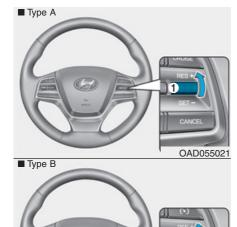
Push the toggle switch (1) up (RES+). If the vehicle speed is over 30 km/h (20 mph), the vehicle will resume the preset speed.
