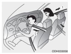
Your vehicle is equipped with driver's and front passenger's Pre-tensioner Seat Belts. The purpose of the pre-tensioner is to make sure the seat belts fit tightly against the occupant's body in certain frontal collisions. The pre-tensioner seat belts may be activated in crashes where the frontal collision is severe enough, together with the air bags.
