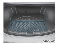
To keep items from shifting in the cargo area, you can use the four holders located in the cargo area to attach the luggage net.
