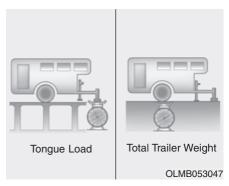
What is the maximum safe weight of a trailer? It should never weigh more than the maximum trailer weight with trailer brakes. But even that can be too heavy. It depends on how you plan to use your trailer. For example, speed, altitude, road grades, outside temperature and how often your vehicle is used to pull a trailer are all important. The ideal trailer weight can also depend on any special equipment that you have on your vehicle.
