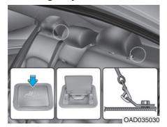
Child Restraint hook holders are located on the package tray.
