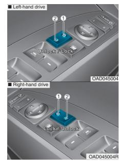
When pressing the (1) portion (1) of the switch, all vehicle doors will lock.
