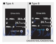
At the end of each driving cycle, the Driving Info message is displayed. This display shows the trip distance (1), the average fuel economy (2), and the remaining distance to empty (3).
