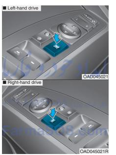
The driver can disable the power window switches on the rear passengers' doors by pressing the power window lock switch.
