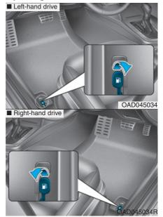
The fuel filler door must be opened from inside the vehicle by pulling up the fuel filler door opener.
