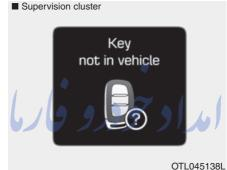
This warning message is displayed if the smart key is not in the vehicle when you press the Engine Start/Stop button.
