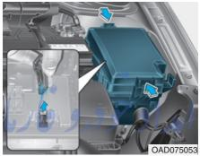
Before inspecting a fuse, you should turn OFF the engine as well as the other electric system switches. If a fuse is blown out, remove the blownout fuse and install a new fuse of the same capacity by using the fuse puller, which is prepared inside the fuse box in the engine compartment. A new fuse may be prepared along with the fuse puller. However, if not, you may temporarily select/use a fuse of the other systems, which do not affect the vehicle operation, such as the audio system.
