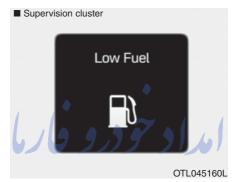
This warning message is displayed if the fuel tank is almost out of fuel.
