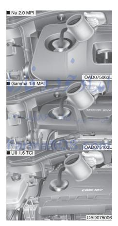
If it is near or at L, add enough oil to bring the level to F. **Do not overfill.**
