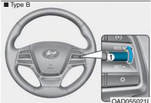
Push the toggle switch (1) up (RES+) and hold it, while monitoring the SET speed on the instrument cluster. Release the toggle switch when the desired speed is shown and the vehicle will accelerate to that speed.
