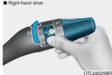
Fog lamps are used to provide improved visibility when visibility is poor due to fog, rain or snow, etc. Use the switch next to the headlamp switch to turn the fog lamps ON and OFF.
