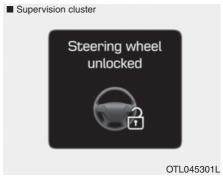
This warning message is displayed if the steering wheel does not lock while the Engine Start/Stop button changes to the OFF position.
