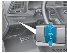
When the vehicle's parking lights or headlights are on, press the illumination control button to adjust the brightness of the instrument panel illumination.
