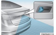
The Rear View Camera will activate when the engine is running and the shift lever is in the R (Reverse) position
