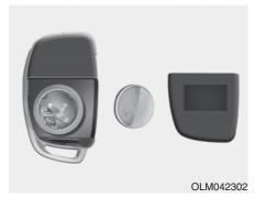
Battery Type: CR2032 To replace the battery:
