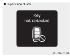
This warning message is displayed if the smart key is not detected when you press the Engine Start/Stop button.
