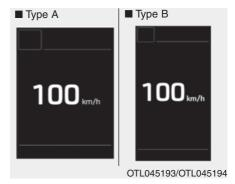
This message shows the speed of the vehicle (km/h, MPH).
