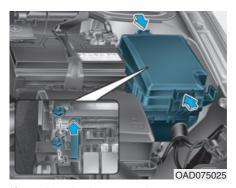
If an electrical system does not operate with no blown fuse in the engine room and inner fuse box, the main fuse inside the battery (+) cap may be blown.
