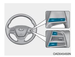
To change the trip mode, press the TRIP button on the steering wheel.
