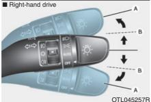
To signal a turn, push down on the lever for a left turn or up for a right turn in position (A). To signal a lane change, move the turn signal lever slightly and hold it in position (B).
