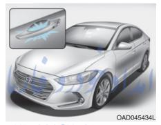
Door handle lamp (if equipped) When all the doors (and trunk) are closed and locked, the door handle lamp will come on for about 15 sec-
