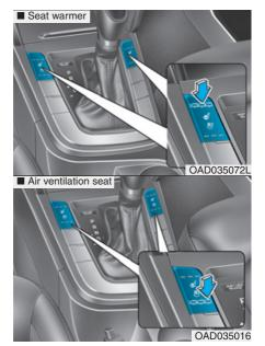
The seat warmers and air ventilation seats are provided to warm or cool the front seats by blowing air through small vent holes on the surface of the seat cushions and seatbacks.
