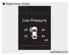
This warning message is displayed if the tire pressure is low. The corresponding tire on the vehicle will be illuminated.
