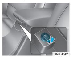
The USB charger is located inside the console box between the driver's seat and the front passenger's seat. Insert the USB charger into the USB port, and re-charge a smart phone or a tablet PC.
