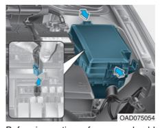
Before inspecting a fuse, you should turn OFF the engine as well as the other electric system switches. If a fuse is blown out, remove the blownout fuse and install a new fuse of the same capacity. Pay extreme caution not to damage the blown-out fuse while removing it.
