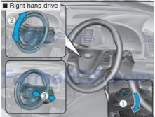
Pull down the lock-release lever (1) on the steering wheel column and adjust the steering wheel angle (2) and position (3, if equipped). Move the steering wheel, so it points toward your chest, not toward your face. Make sure you can see the instrument panel warning lights and gauges.
