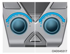
Turn the temperature control knob to set the desired temperature.
