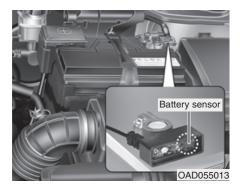
The battery sensor is deactivated, when the battery is disconnected from the negative pole for maintenance purpose.
