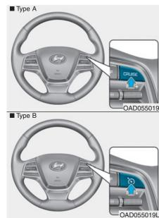
Press the CRUISE / (S) button on the steering wheel to turn the system on. The CRUISE indicator will illuminate.
