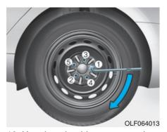
13. Use the wheel lug nut wrench to tighten the lug nuts in the order shown. Double-check each lug nut until they are tight. After changing tires, we recommend that an authorized HYUNDAI dealer tighten the lug nuts to their proper torque as soon as possible. The wheel lug nut should be tightened to 11~13 kgf.m (79~94 lbf.ft).
