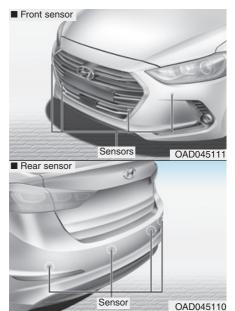
The Parking Assist System assists the driver during movement of the vehicle by chiming if any object is sensed within approximately 100 cm (40 in) in front and 120 cm (47 in) behind the vehicle.
