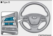
The steering wheel audio control button is installed for your convenience.
