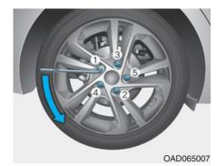
Loosen the wheel lug nuts counterclockwise one turn each in the order shown above, but do not remove any lug nuts until the tire has been raised off of the ground.
