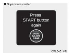
This message is displayed if you were unable to start the vehicle when the Engine Start/Stop button was pressed.
