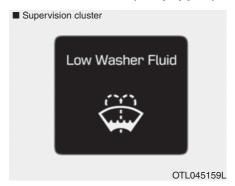
This warning message is displayed in the service reminder mode if the washer fluid level in the reservoir is nearly empty.
