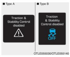
Press and hold the ESC OFF button continuously for more than 3 seconds. The ESC OFF indicator light and message (vehicles equipped with a supervision cluster) illuminates and a warning chime sounds. In this state, both the traction control function of ESC (engine management) and the brake control function of ESC (braking management) are disabled.
