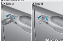
Turn the key toward the rear of the vehicle to unlock and toward the front of the vehicle to lock
