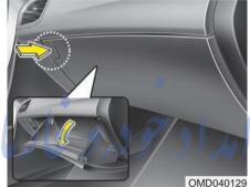
To open the glove box, push the button and the glove box will automatically open.
