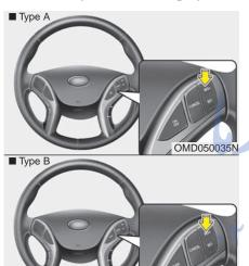
Push the RES+ switch. If the vehicle speed is over 20 mph (30 km/h), the vehicle will resume the preset speed.
