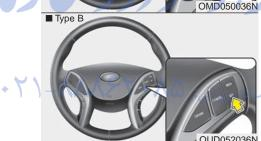
Lightly tap the brake pedal. When the vehicle attains the desired speed, push the SET- switch.
