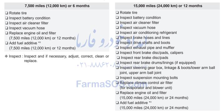
\* Inspect : Inspect and if necessary, adjust, correct, clean or replace.
