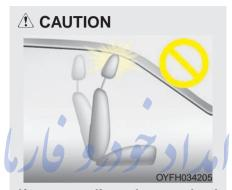
If you recline the seatback towards the front with the headrest and seat cushion raised, the headrest may come in contact with the sunvisor or other parts of the vehicle.
