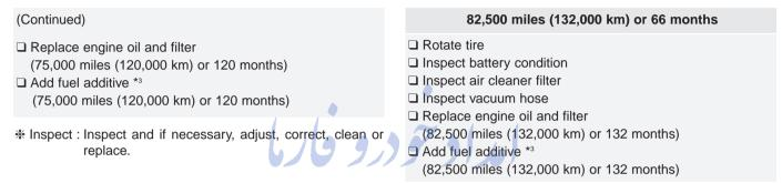
\* Inspect : Inspect and if necessary, adjust, correct, clean or replace.
