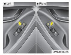
While the engine is running, push either switch to warm the rear seat.
