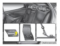
First, secure the child restraint with the LATCH lower anchors or the seat belt. If the child seat manufacturer recommends that the tether strap be attached, attach and tighten the tether strap to the tether anchor.
