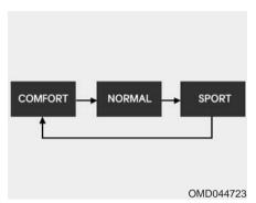
When the steering mode button is pressed, the selected steering mode will appear on the cluster.
