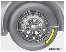
14. Use the wheel lug nut wrench to tighten the lug nuts in the order shown. Double-check each lug nut until they are tight. After changing tires, we recommend that an authorized HYUNDAI dealer tighten the lug nuts to their proper torque as soon as possible. The wheel lug nut should be tightened to 65~79 lb.ft (9~11 kg.m).
