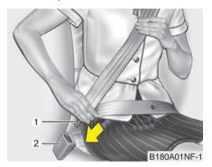
Pull the seat belt out of the retractor and insert the metal tab (1) into the buckle (2). There will be an audible "click" when the tab locks into the buckle.
