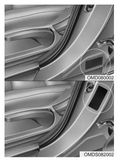
The vehicle certification label attached on the driver's side center pillar gives the Vehicle Identification Number (VIN).
