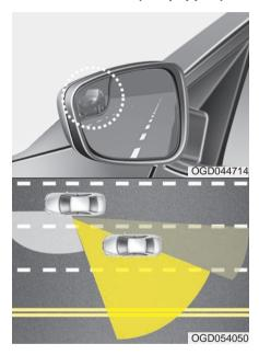
The Blind zone mirror (BZM) is a supplemental mirror that reduces the driver's blind zone by showing the rear side area of the vehicle. The blind zone mirror is equipped on the left-hand outside rearview mirror
