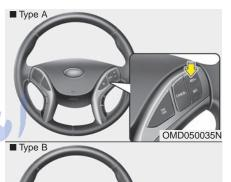
Push the RES+ switch and hold it, while monitoring the SET speed on the instrument cluster. Release the switch when the desired speed is shown and the vehicle will accelerate to that speed.
