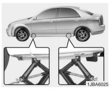
8. Place the jack at the designated jacking position under the frame closest to the tire you are changing. The jacking positions are plates welded to the frame with two tabs and a raised dot. Never jack any other position or part of the vehicle.
