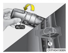
When the light switch is in the AUTO position, the parking (position) light and headlights will be turned ON or OFF automatically depending on the amount of light outside the vehicle.
