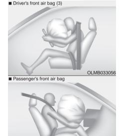
After complete inflation, the air bag immediately starts deflating, enabling the driver to maintain forward visibility and the ability to steer or operate other controls.
