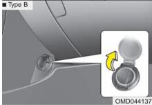
The power outlet is designed to provide power for mobile telephones or other devices designed to operate with vehicle electrical systems. The devices should draw less than 15 amps with the engine running.
