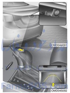
The rearview camera will activate when the back-up light is ON with the engine start/stop button ON and the shift lever in the R position.
