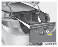
3. Pull on the seatback folding lever located in the trunk.
