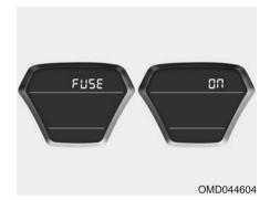
This warning message illuminates if the fuse switch under the steering wheel is OFF.
