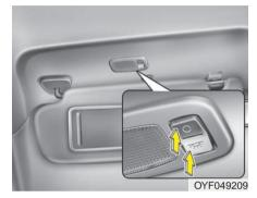
Push the switch to turn the light ON or OFF.
