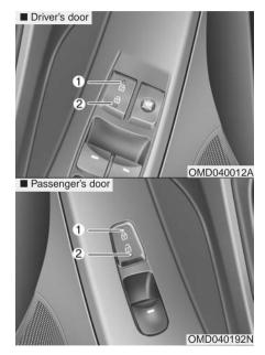
When pressing the  $(\frac{1}{2})$  portion (1) of the switch, all vehicle doors will lock.
