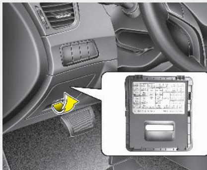
Inner panel fuse panel
