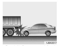
Frontal Air Bags may not inflate in "under-ride" collisions where the collisions energy is absorbed above the vehicle's front bumper.
