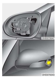
Unscrew the bolt with a cross-tip screwdriver and then remove the lens from the housing.
