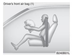
The air bag modules are located both in the center of the steering wheel and in the front passenger's panel above the glove box. When the SRSCM detects a sufficiently severe impact to the front of the vehicle, it will automatically deploy the front air bags.
