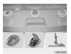
Securing a child restraint seat with "Tether Anchor" system
