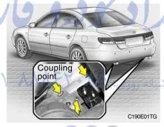
5. The maximum permissible overhang of the coupling point is 1,255 mm.
