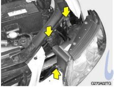
4. Using a spanner of the correct size, remove the headlight assembly mounting bolts and nut.
