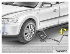
Lower the car to the ground by turning the wheel nut wrench counterclockwise.
