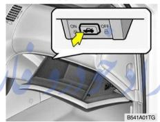
The trunk lid control button located in the vehicle glove box is used to prevent unauthorized access to the trunk. above and leave the sub key with the attendent. Sub key can start the engine and operate door locks only.
