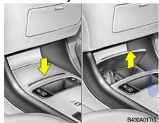
The front ashtray may be opened by pushing and releasing the ashtray lid. To clean the ashtray, the plastic receptacle should be removed by lifting the plastic ash receptacle upward and pulling it out. The ashtray light will only illuminate when the external lights are FarmaSOS.com on.
