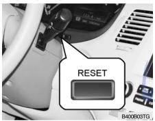
Push in the RESET switch more than 1 second to initialize the displayed information such as tripmeter, average speed, drive time and average fuel consumption.
