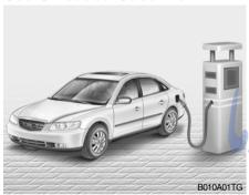
Unleaded gasoline with a Pump Octane Rating of 87 (Research Octane Number 91) or higher must be used in Hyundai vehicle. If leaded gasoline is used, it will cause the catalytic converter to become ineffective and the emission control system to malfunction.
