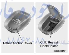
1. Open the tether anchor cover on the rear seat package tray.
