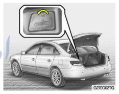
2. Remove the cover on the inside of rear luggage trim by turning the knob counterclockwise.
