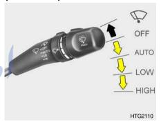
When the windshield wiper switch is placed in the "AUTO" position, the rain sensor located on the upper end of windshield glass senses the amount of rainfall and controls for the appropriate length of the intervals between wipes appropriately.
