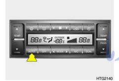
The FATC (Full Automatic Temperature Control) system automatically controls the heating and cooling by doing as follows:
