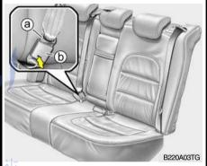
o To disconnect the metal tab (a) from the buckle (b), insert a narrow-ended tool into the groove located on the buckle (b).
