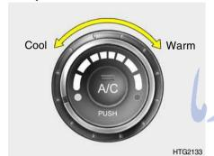
This control is used to adjust the degree of heating or cooling desired.
