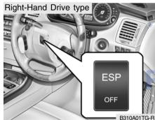
The Electronic Stability Program (ESP) system is designed to stabilize the vehicle during cornering maneuvers.
