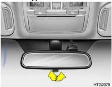
Your Hyundai is equipped with a day/ night inside rearview mirror. The "night" position is selected by flipping the tab at the bottom of the mirror toward you. In the "night" position, the glare of headlights of cars behind you is reduced.
