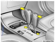
The highly efficient Hyundai automatic transaxle has five forward speeds and one reverse speed. The individual speeds are selected automatically, depending on the position of the speed selector lever. The selector lever has 2 gates; the main gate and the manual gate.
