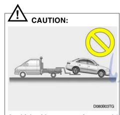
A vehicle with an automatic transaxle should never be towed from the rear with the front wheels on the ground. This can cause serious damage to the transaxle. Be sure to use a towing dolly under the front wheels.
