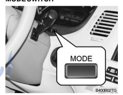
Pushing in the MODE switch when the ignition switch is in "ON" position changes the display as follows;
