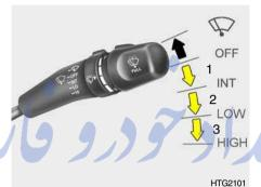
The windshield wiper switch has three positions:
