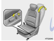
Pull the upper portion of the control knob forward or backward to recline the seatback to the desired position. Release the control knob and the seatback will remain in that position.
