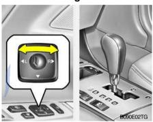
While the vehicle is moving backward, the outside rearview mirror(s) will move downward to aid reverse parking safely. According to the position of the outside rearview mirror switch knob, the outside rearview mirror(s) will operate as follows.
