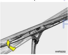
1. Put a new wiper blade onto the wiper arm and lower the wiper blade at the level of the wiper arm as shown in the drawing.
