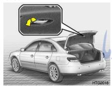
Your vehicle is equipped with a glowin-the dark emergency trunk release lever located inside the trunk. It will glow after the trunk is closed. When pulled, this lever will release the trunk latch mechanism and open the trunk.
