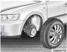
Use the wrench to loosen the wheel nuts, then remove them with your fingers. Slide the wheel off the studs and lay it flat so it cannot roll away. To put the wheel on the hub, pick up the spare tire, line up the holes with the studs and slide the wheel onto them. If this is difficult, tip the wheel slightly and get the top hole in the wheel lined up with the top stud. Then jiggle the wheel back and forth until the wheel can be slid over the other studs.
