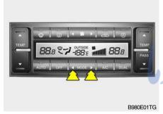
This is used to direct the flow of air. Air can be directed to the floor, dashboard outlets, or windshield. Four symbols are used to represent Face, Bi-Level, Floor and Floor-Defrost air position.
