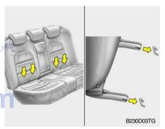
To engage the child restraint seat to the ISOFIX anchor, insert the child restraint seat latch into the ISOFIX anchor. Listen for the audible "click" sound.  Connect the tether strap hook to the child restraint hook holder and tighten to secure the seat. Refer to "Securing a Child Restraint System With Tether Anchorage System" on page 1-40.
