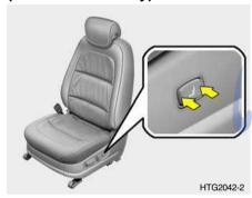
To adjust the lumbar support, press the control switch the outboard side of the seat cushion. To increase the amount of lumbar support, press the front portion of the switch. To decrease it, press the rear portion of the switch.
