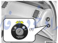
The passenger's front airbag can be deactivated by the passenger's front airbag ON/OFF switch (1) if a child restraint is installed on the front passenger's seat or if the front passenger's seat is unoccupied by a person.
