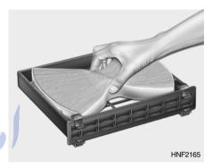
5. Replace the air conditioner filter by lifting it.
