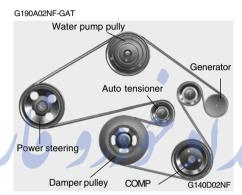
Drive belts should be checked periodically for proper tension. At the same time, belts should be examined for cracks, wear, fraying or other evidence of deterioration and replaced if necessary.
