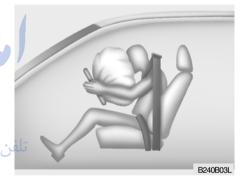
A fully inflated airbag in combination with a properly worn seat belt slows the driver's or the passenger's forward motion, thus reducing the risk of head or chest injury.
