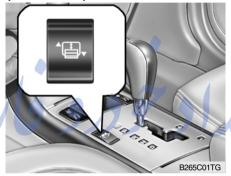
Press the curtain switch to raise the rear window curtain. To lower the rear window curtain, press the switch once again.
