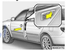
The doors can be locked without a key. To lock the doors from the outside, first push the inside lock switch to the "LOCK" position, so that the red mark on the switch is not visible, then close the door.
