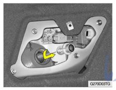
3. To replace the turn signal light, remove it from the bulb holder and install the new bulb.
