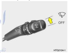
If a single wipe is desired in mist, push the windshield wiper and washer control lever upwards. 82
