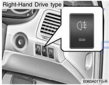
To turn on the rear fog lights, push the switch. They will light when the headlight switch is in the first position and the key is in the "ON" position.
