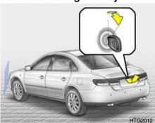
To open the trunk lid, insert the key and turn it clockwise to unlock. The trunk compartment light comes on when the trunk lid is opened.
