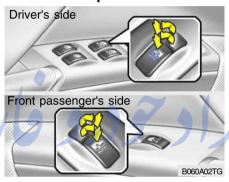
The auto up/down window is controlled by the window switch on the driver's and front passenger's armrest.
