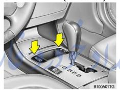
The front seats can be electrically heated individually when the ignition switch is ON. When the switch is ON, a number ranging from 1 to 5 is displayed on the switch (5 = warmest setting). To turn off the seat warmer, set the switch to 0.
