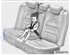
Use the center seat belt for the rear to secure the child restraint system as illustrated. After installation of the child restraint system, rock the child seat back and forth, and side to side to ensure that it is properly secured by the seat belt.
