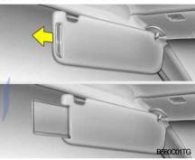
Your vehicle is equipped with sun visor extenders that may be used when the visor is in the side glass position.
