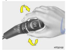
To use the intermittent wiper feature, place the wiper switch in the "INT" position. With the switch in this position, the interval between wipes can be varied from approximately 1 to 18 seconds by turning the interval adjuster barrel. This is also varied automatically depending on your road speed.
