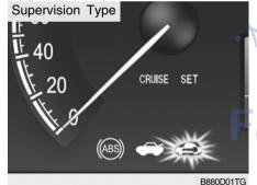
In case the immobilizer warning indicator blinks for five seconds when the ignition key is turned to "ON" position, this indicates that the immobilizer system is out of order. And you cannot start the engine without the limp home procedures with ignition key.
