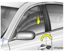
To open the windows, turn the key toward the rear of the vehicle for 3 seconds.
