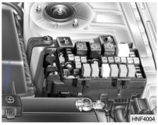
A fusible link will melt if the electrical circuits from the battery are ever overloaded, thus preventing damage to the entire wiring harness. (This could be caused by a short in the system drawing too much current.) If this ever happens, have a Hyundai dealer determine the cause, repair the system and replace the fusible link. The fusible links are located in a relay box for easy inspection.
