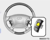
The vehicle will automatically resume the speed set prior to cancellation when you push the control switch "RESUME (ACCEL)" and release it to return (when travelling above 40 km/h).
