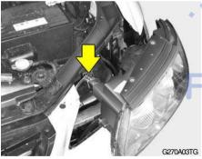
5. Disconnect the power cord from the back of the headlight.
