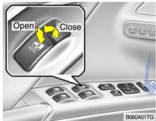
The power windows operate when the ignition key is in the "ON" position. The main switches are located on the driver's armrest and control the front and rear windows on both sides of the vehicle. The windows may be opened by depressing the appropriate window switch and closed by pulling up the switch. To open the window on the driver's side, press the switch halfway down. The window moves as long as the switch is operated.
