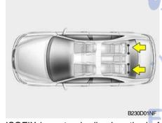
ISOFIX is a standardized method of fitting child seats that eliminates the need to use the standard adult seat belt to secure the seat in the vehicle. This enables a much more secure and positive location with the added benefit of easier and quicker installation.
