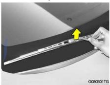
1. Place the windshield wiper switch to the "OFF" position, raise the windshield wiper arm about 10 mm from the windshield as illustrated.
