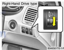
To adjust the headlight beam level according to the number of the passengers and the loading weight in the luggage area, turn the beam leveling switch.
