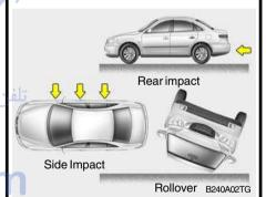
o Front airbags are not intended to deploy in side-impact, rear-impact or rollover crashes. In addition, airbags will not deploy in frontal crashes below the deployment threshold speed.
