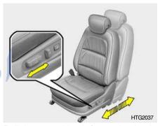
Pull the control knob forward or backward to move the seat forward or backward to the desired position. Release the control knob and the seat will remain at that position. B090D01NF-GAT
