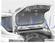
2. Loosen the mounting screws of the trunk lid trim with a phillips screwdriver and remove the trunk lid trim.
