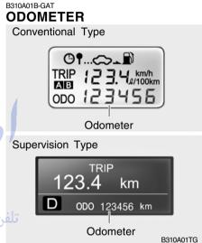
The odometer records the total driving distance in kilometers or miles, and is
