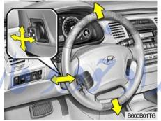
To adjust the desired position of the steering wheel, operate the adjusting switch on the left side of the steering wheel.
