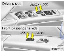
The central door locking switch is located on the driver's and front passenger's armrest. It is operated by depressing the door lock switch. If any door is open when the switch is depressed to the "LOCK" position, the door will remain locked when closed. FarmaSOS.cor
