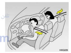
When the vehicle stops suddenly, or if the occupant tries to lean forward too quickly, the seat belt retractor will lock into position. In certain frontal collisions, the pretensioner will activate and pull the seat belt into tighter contact against the occupant's body. The buckle pretensioner (which is installed in the buckle) will also pull the seat belt into the buckle.
