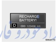
If your vehicle is equipped with the supervision type cluster, the warning text is double informed on the dot matrix display.
