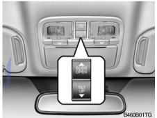
If your vehicle is equipped with this feature, you can slide or tilt your sunroof with the sunroof control buttons located on the overhead console.
