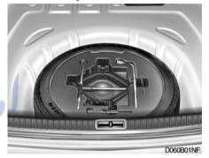
Take out the tool receptacle and turn the installation bolt counterclockwise to obtain spare tire from the trunk.
