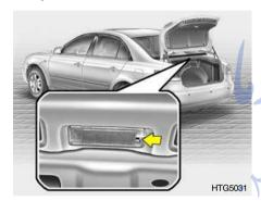
2. Remove the luggage compartment light cover on the rear package tray panel with a blade screwdriver.
