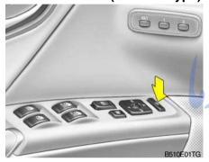
Both left and right outside rearview mirrors can be folded by pressing the outside rearview mirror folding switch. The outside rearview mirrors can be folded rearward for parking in narrow areas.
