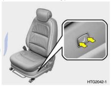
To adjust the lumbar support, press the control switch on the outboard side of the seat cushion. To increase the amount of lumbar support, press the front portion of the switch. To decrease it, press the rear portion of the switch.
