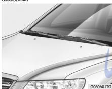
The wiper blades should be carefully inspected from time to time and cleaned to remove accumulations of road film or other debris. To clean the wiper blades and arms, use a clean sponge or cloth with a mild soap or detergent and water. If the wipers continue to streak or smear the glass, replace them with genuine Hyundai replacement parts or their equivalent.
