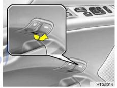
To open the trunk lid without using the key, pull up the lid release lever.
