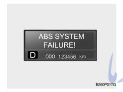
If your vehicle is equipped with the supervision type cluster, the warning text is double informed on the dot matrix display. The warning text comes on for about 20 seconds. If you push the RESET button behind the steering wheel, the warning text will go out.
