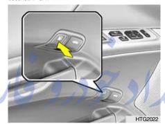
The fuel-filler lid may be opened from inside the vehicle by pushing on the fuel-filler lid opener located on the driver side door.
