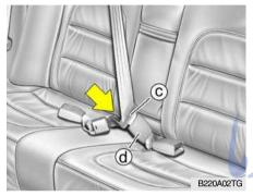
3. After confirming that (a) and (b) are latched, pull the seat belt out of the retractor and insert the metal tab (c) into the buckle (d).
