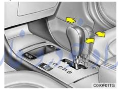
Whether the vehicle is stationary or in motion, sports mode is selected by pushing the selector lever from the "D" position into the manual gate. To return to "D" range operation, push the selector lever back into the main gate. In sports mode, moving the selector lever backwards and forwards can make rapid gearshifts simple. In contrast to a manual transaxle, the sports mode allows gearshifts with the accelerator pedal depressed.
