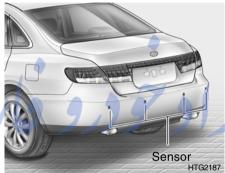
The back warning system assists the driver during backward movement of the vehicle by chiming if any object is sensed within the distance of 1200 mm (47 in.) behind the vehicle. This system is only a supplemental system.
