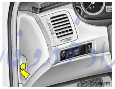
The fuse box for the lights and other electrical accessories will be found in the left side of the crash pad. Inside the box you will find a list showing the circuits protected by each fuse. If any of your car's lights or other electrical accessories stop working, a blown fuse could be the reason. If the fuse has burned out, you will see that the metal strip inside the fuse has burned through. If you suspect a blown fuse, follow this procedure:
