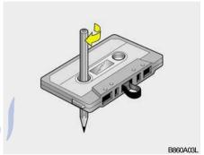
Look at a tape before you insert it. If the tape is loose, tighten it by turning one of the hubs with a pencil or your finger.
