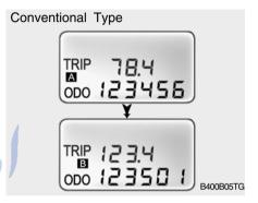
To shift from TRIP A to TRIP B, press the TRIP switch.
