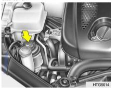
The power steering fluid level should be checked regularly.
