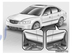
The base of the jack should be placed on firm, level ground. The jack should be positioned as shown in the drawing.
