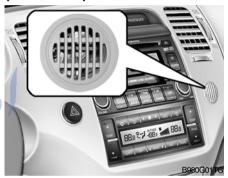
There is a humidity sensor on the center fascia panel. If it becomes very humid inside the car, the air conditioning is turned on automatically to control the humidity.
