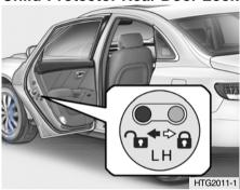
Your Hyundai is equipped with a "childprotector" rear door lock assembly. When the lock mechanism is engaged, the rear door cannot be opened from the inside. Its use is recommended whenever there are small children in the rear seat.
