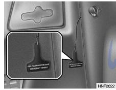
If the fuel filler lid cannot be opened using the remote opener, a manual opener handle is located inside the trunk on the left side. Open the fuel filler lid by pulling on this handle as shown in the illustration.
