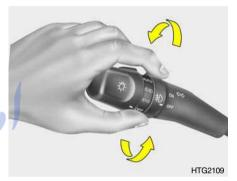
To turn on the front fog lights, place the switch in the "ON" position. They will light when the headlight switch is in the first position.
