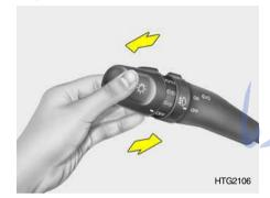
To turn on the headlight high beams, push the lever forward (away from you). The High Beam Indicator Light will come on at the same time. For low beams, pull the lever back toward you.
