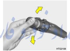
To indicate a lane change, move the lever up or down to a point where it begins flashing. • 🔨 🔾 : ....
