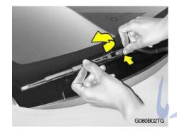
2. Remove the windshield wiper blade with the "LOCK" lever pressed.
