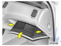
3. Lower the glove box down completely by pushing both sides of the glove box inward.
