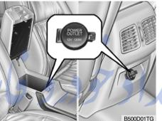
These supply 12V electric power to operate electric accessories or equipment only when the key is in the "ON" or "ACC" position.
