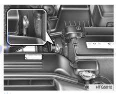
2. Remove the transaxle dipstick, wipe it clean, reinsert the dipstick as far as it will go, then remove it again. Now check the fluid level on the dipstick. It should be in the "HOT" range on the dipstick.
