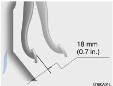
You need a helper to check the brake pedal clearance. With the engine running, have your helper press down on the brake pedal several times and then hold it down with a force of about 490N (50 kg, 110 lbs). The brake pedal clearance is the distance from the top surface of the brake pedal to the asphalt sheeting under the floor mat. If the brake pedal clearance is not within the limits specified in the illustration, have it inspected by your Hyundai dealer and adjusted or repaired if necessary.
