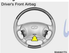
Your Hyundai is equipped with a Supplemental Restraint (Airbag) System. The indications of the system's presence are the letters "SRS AIR BAG" embossed on the airbag pad cover in the steering wheel and the front passenger's panel pad above the glove box.
