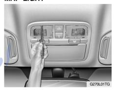
1. Remove the plastic cover with a blade screwdriver.
