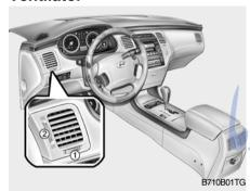
The vents are opened when the vent knob is moved to "  $\leq$  " position. The vents are closed when the vent knob is moved to " , ". Keep these vents clear of any obstructions.
